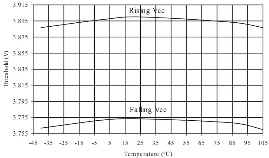
**Figure 35-30 BOD Thresholds vs. Temperature (BOD Level is 2.7V)**
