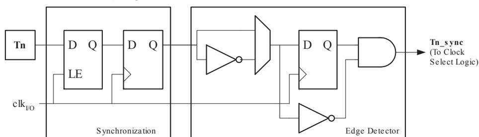
The synchronization and edge detector logic introduces a delay of 2.5 to 3.5 system clock cycles from an edge has been applied to the T3/T2/T1 pin to the counter is updated.
