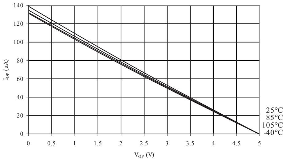
**Figure 35-16 I/O Pin Pull-up Resistor Current vs. Input Voltage (VCC = 2.7V)**
