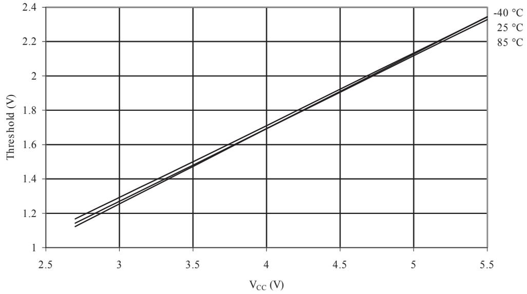
**Figure 34-35 Reset Input Pin Hysteresis vs.  $V_{CC}$**
