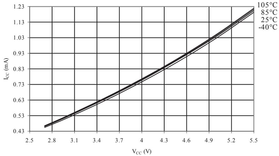
**Figure 35-12 Idle Supply Current vs. V<sub>CC</sub> (Internal RC Oscillator, 1MHz)**
