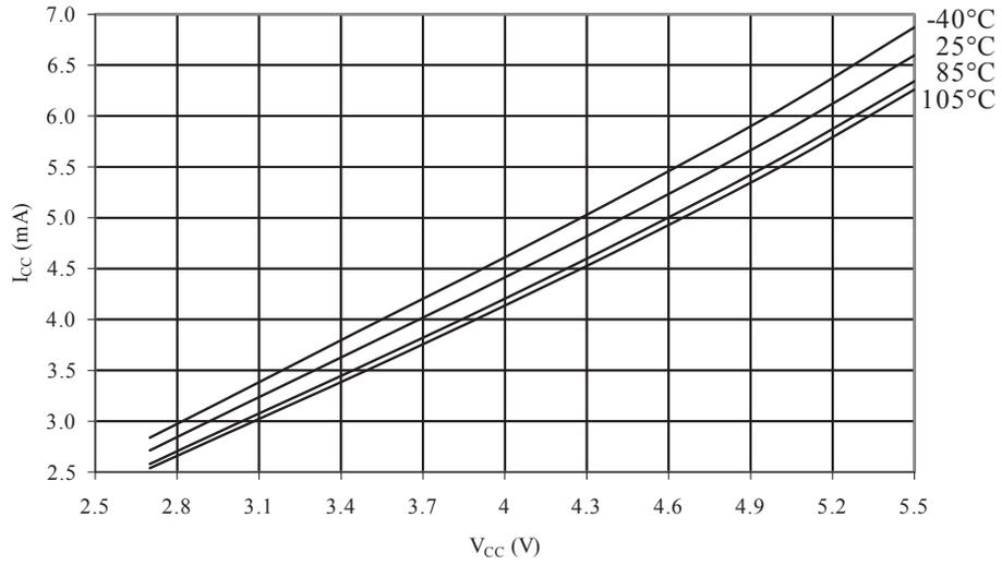
**Figure 35-5 Active Supply Current vs. V<sub>CC</sub> (Internal RC Oscillator, 2MHz)**
