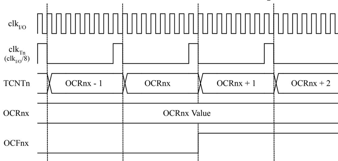
The next figure shows the count sequence close to TOP in various modes. When using phase and frequency correct PWM mode the OCRnx Register is updated at BOTTOM. The timing diagrams will be the same, but TOP should be replaced by BOTTOM, TOP-1 by BOTTOM+1 and so on. The same renaming applies for modes that set the TOVn Flag at BOTTOM.
