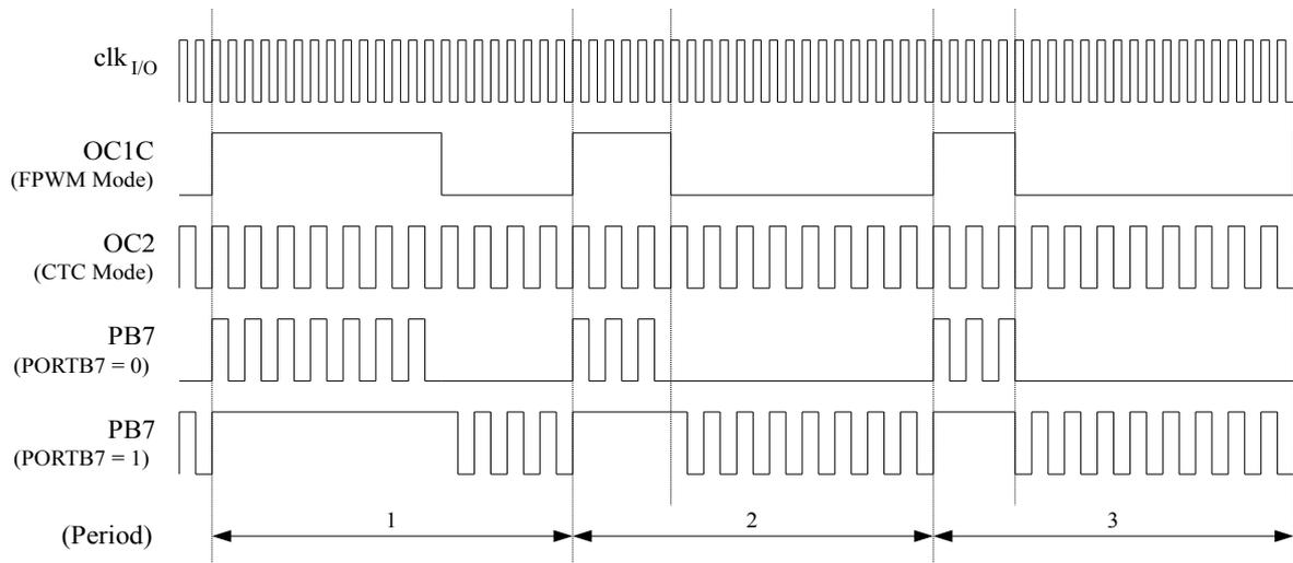
In this example, Timer/Counter2 provides the carrier, while the modulating signal is generated by the Output Compare unit C of the Timer/Counter1.
