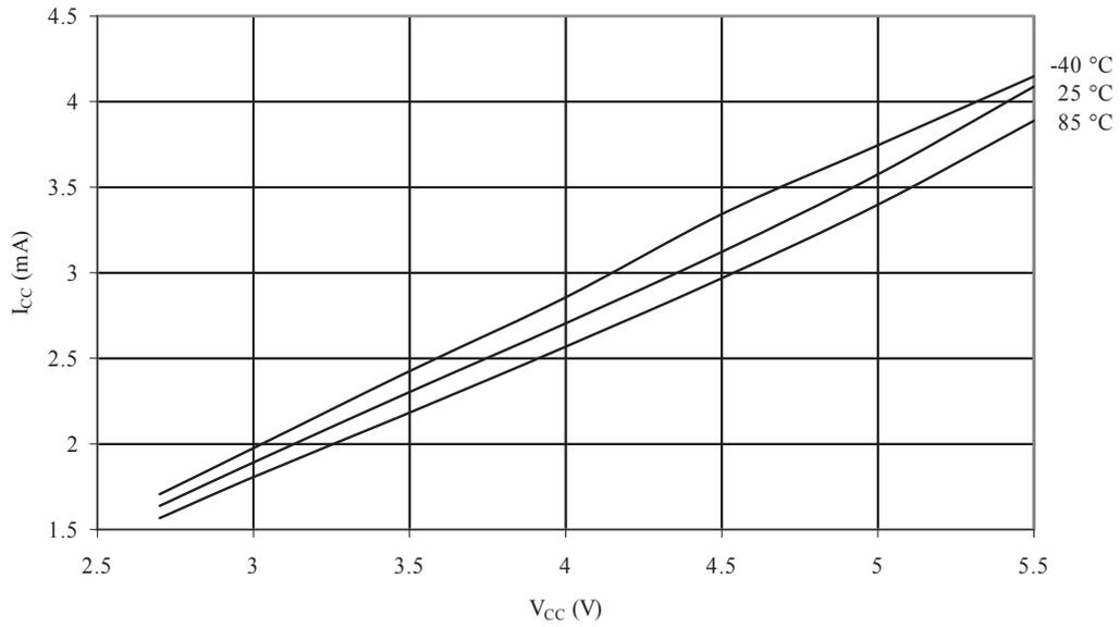
**Figure 34-5 Active Supply Current vs.  $V_{CC}$  (Internal RC Oscillator, 4 MHz)**
