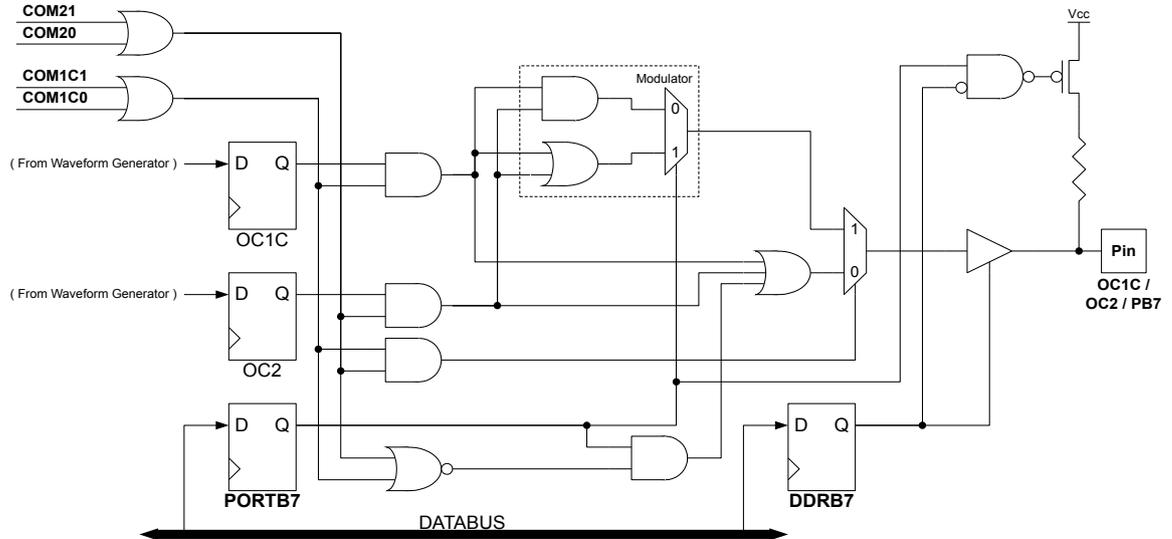
When the modulator is enabled the type of modulation (logical AND or OR) can be selected by the PORTB7 Register. Note that the DDRB7 controls the direction of the port independent of the COMnx1:0 bit setting.
