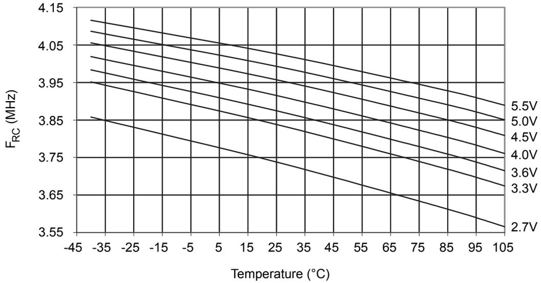
**Figure 35-39 Calibrated 4MHz RC Oscillator Frequency vs.  $V_{CC}$**
