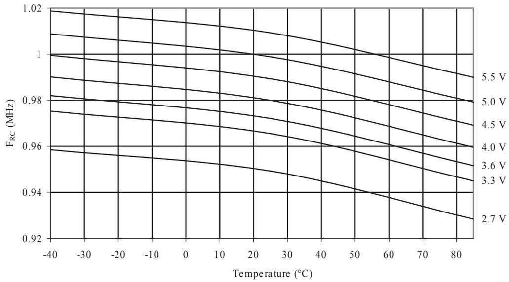
**Figure 34-41 Calibrated 1 MHz RC Oscillator Frequency vs. V<sub>CC</sub>**
