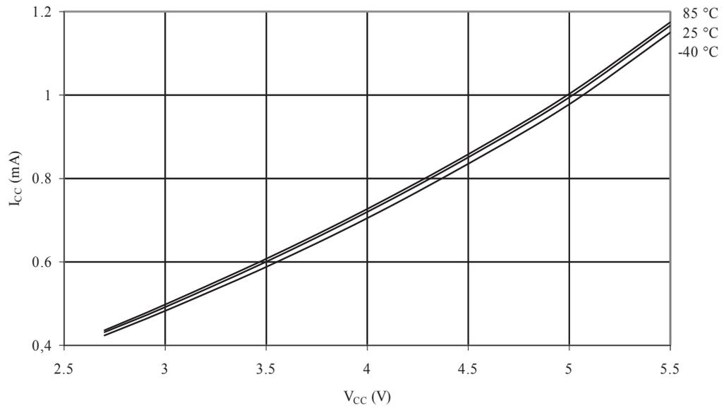
**Figure 34-12 Idle Supply Current vs.  $V_{CC}$  (Internal RC Oscillator, 4 MHz)**
