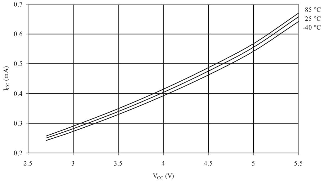
**Figure 34-11 Idle Supply Current vs.  $V_{CC}$  (Internal RC Oscillator, 2 MHz)**
