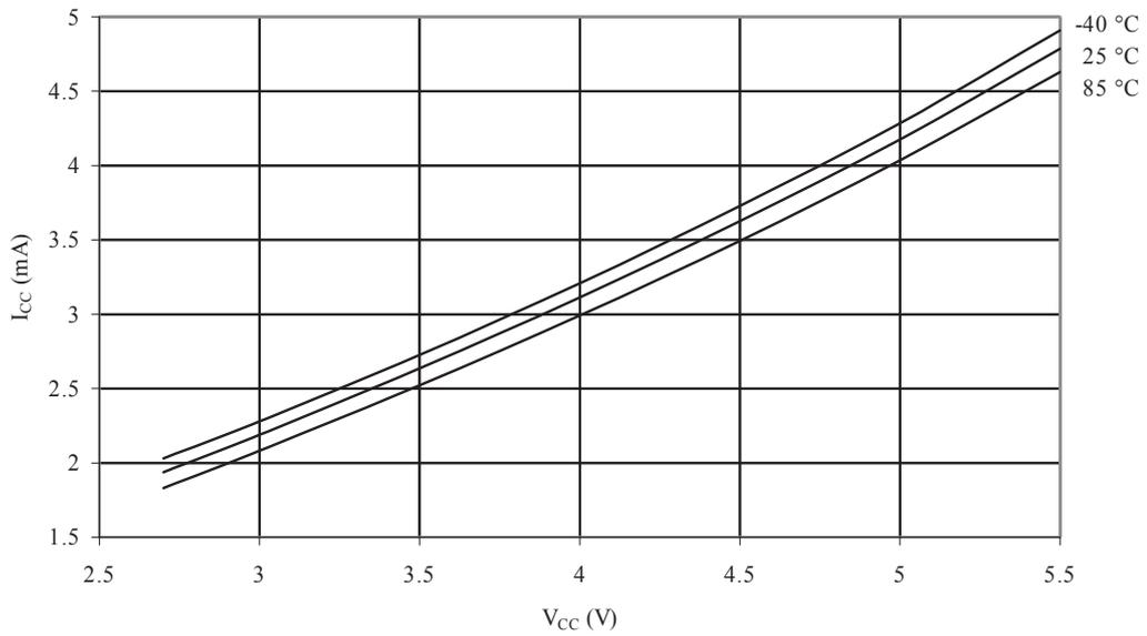
**Figure 34-14 Idle Supply Current vs. V<sub>CC</sub> (32 kHz External Oscillator)**
