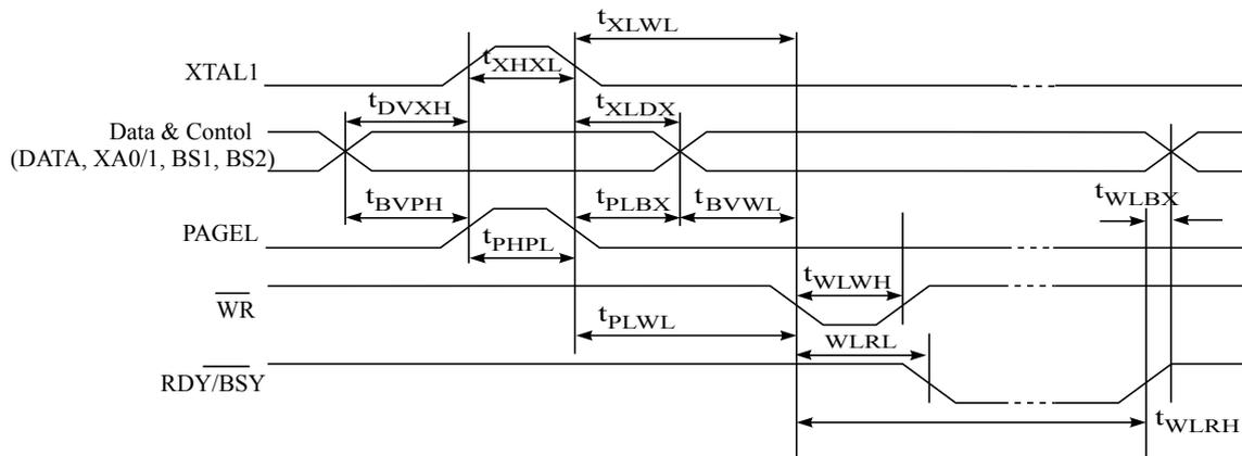
Figure 32-5 Parallel Programming Timing, Loading Sequence with Timing Requirements<sup>(1)</sup>
