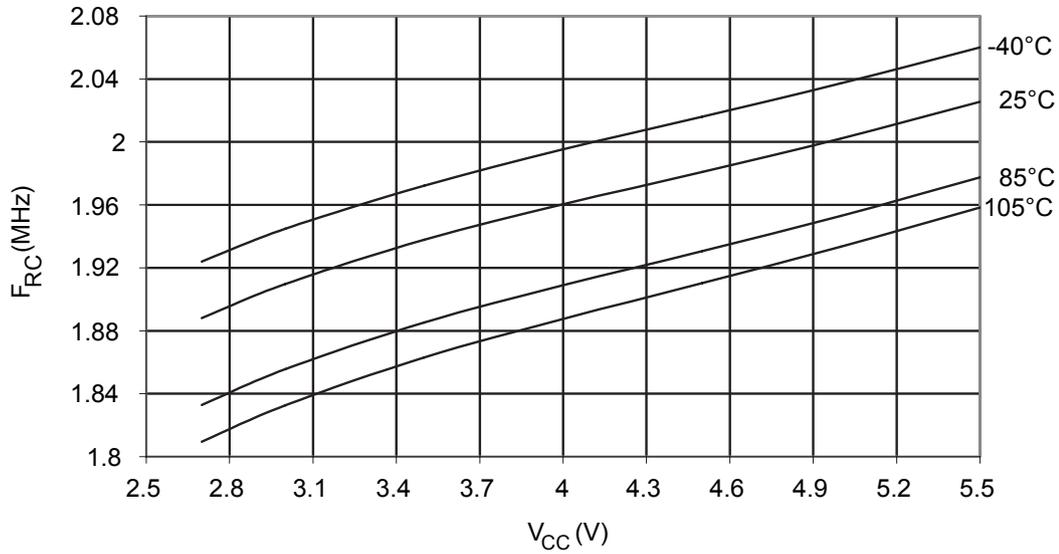
**Figure 35-38 Calibrated 4MHz RC Oscillator Frequency vs. Temperature**
