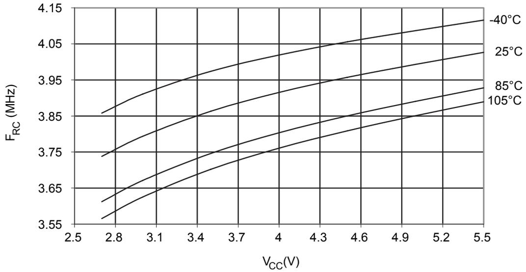
**Figure 35-40 Calibrated 8MHz RC Oscillator Frequency vs. Temperature**
