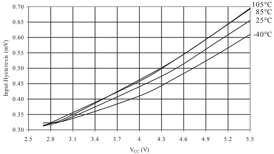
**Figure 35-26 Reset Input Threshold Voltage vs.  $V_{CC}$  ( $V_{IH}$ , Reset Pin Read as "1")**
