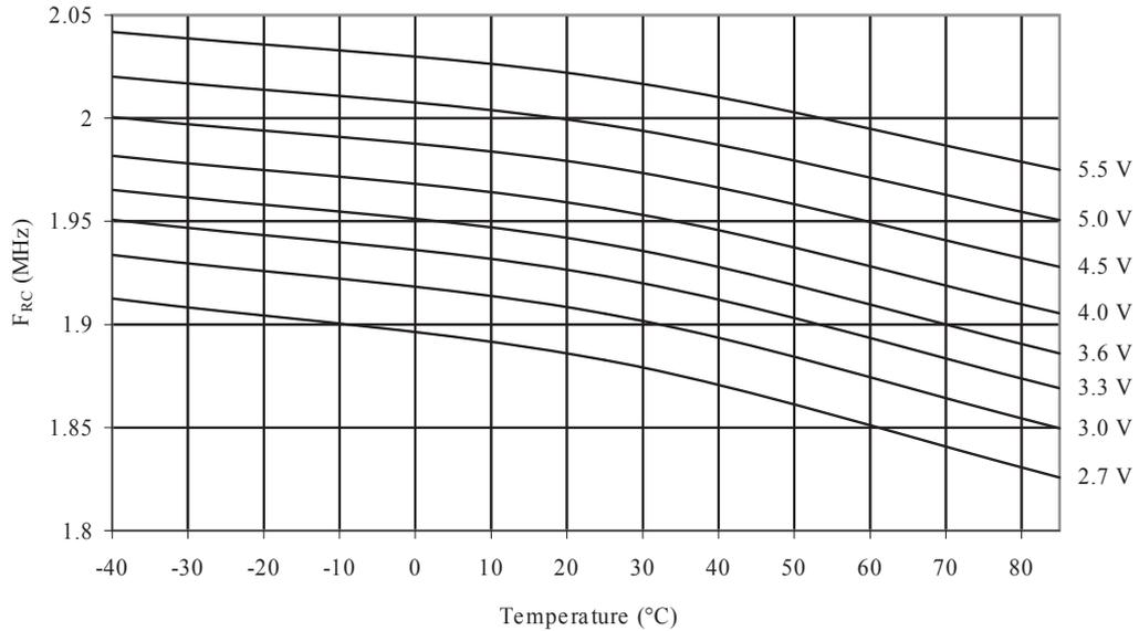
**Figure 34-44 Calibrated 2 MHz RC Oscillator Frequency vs. V<sub>CC</sub>**
