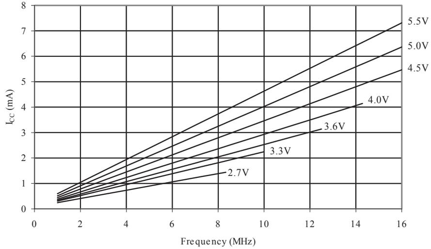
**Figure 35-9 Idle Supply Current vs. V<sub>CC</sub> (Internal RC Oscillator, 8MHz)**
