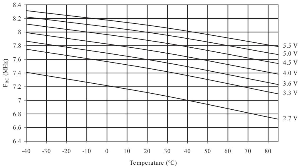
**Figure 34-50 Calibrated 8 MHz RC Oscillator Frequency vs. V<sub>CC</sub>**
