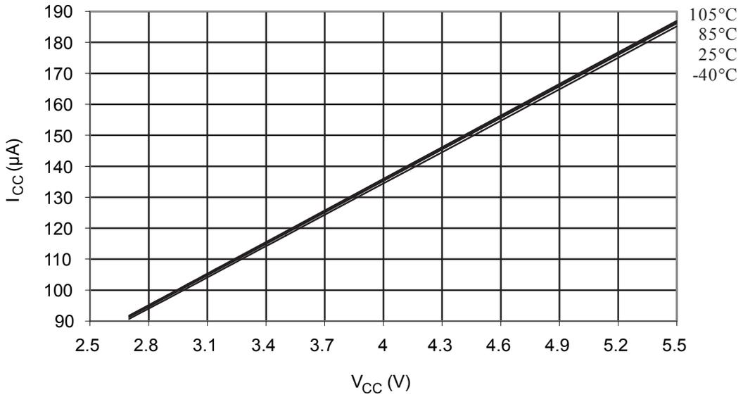
Figure 35-46 Watchdog Timer Current vs.  $V_{CC}$
