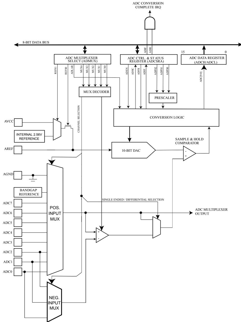
The ADC converts an analog input voltage to a 10-bit digital value through successive approximation. The minimum value represents GND and the maximum value represents the voltage on the AREF pin minus 1 LSB. Optionally, AVCC or an internal 2.56V reference voltage may be connected to the AREF pin by writing to the REFSn bits in the ADMUX Register. The internal voltage reference may thus be decoupled by an external capacitor at the AREF pin to improve noise immunity.
