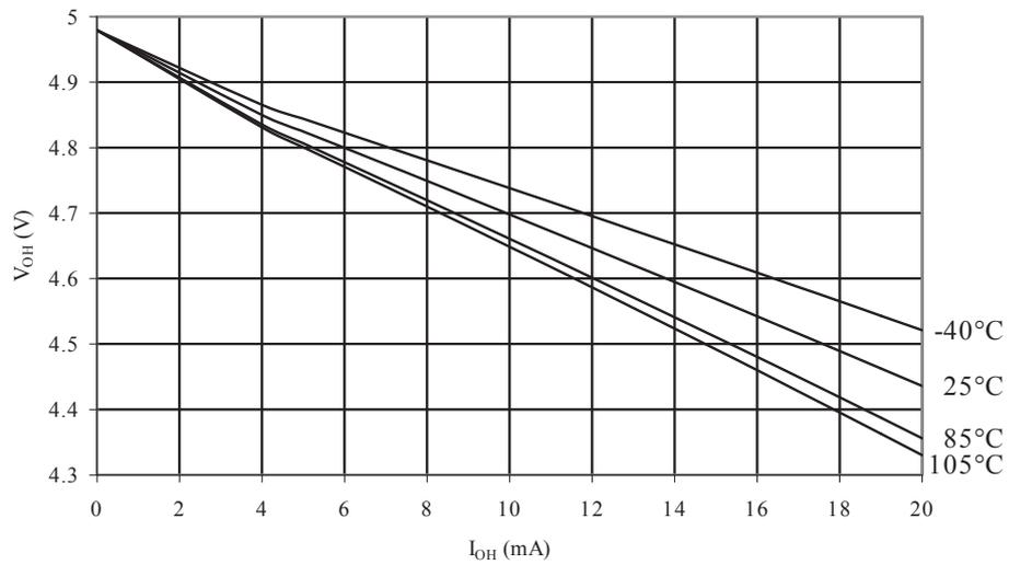
**Figure 35-20 I/O Pin Output Voltage vs. Source Current, Port B ( $V_{CC} = 3V$ )**
