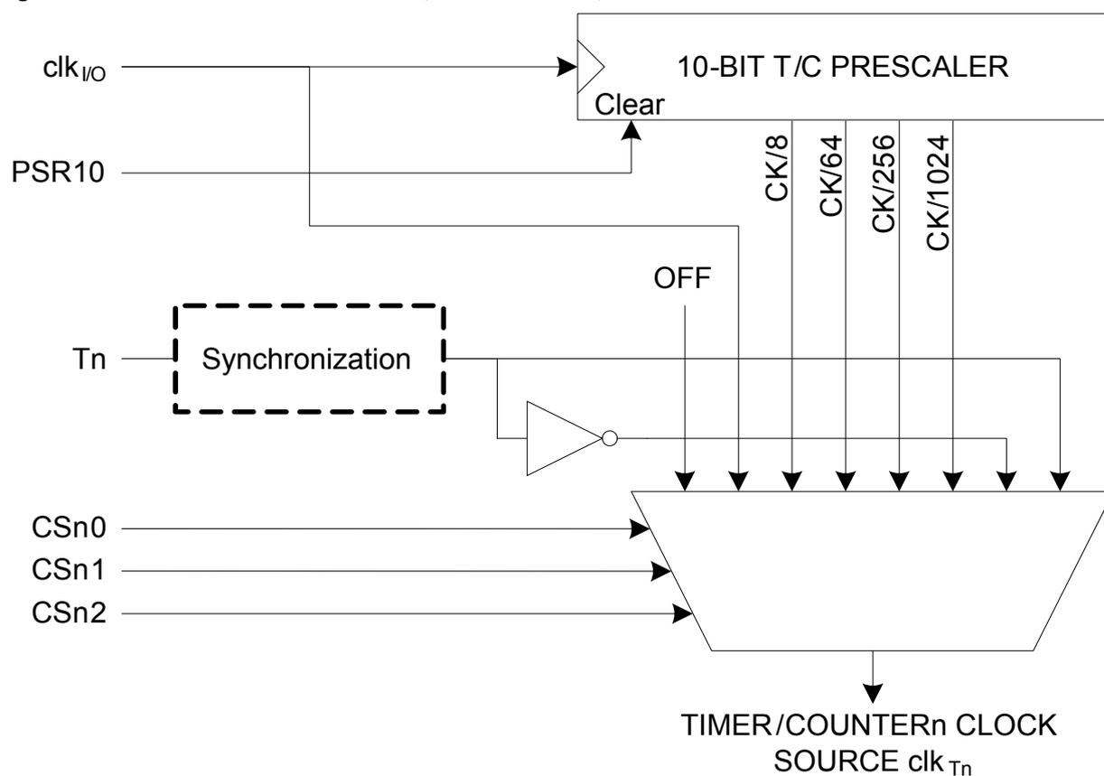
**Note:** 1. The synchronization logic on the input pins (T3/T2/T1) is shown in figure [T3/T2/T1 Pin Sampling](#) in this section.
