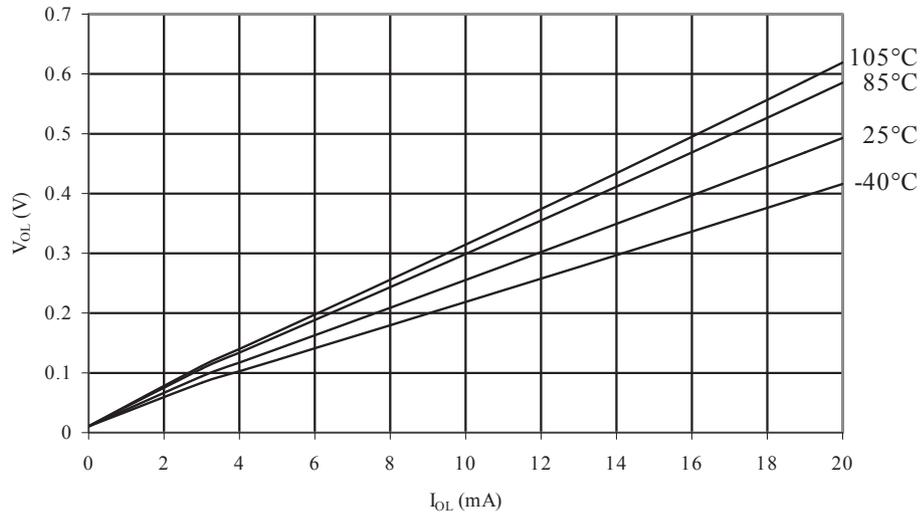
**Figure 35-22 I/O Pin Output Voltage vs. Sink Current, Port B ( $V_{CC} = 3V$ )**
