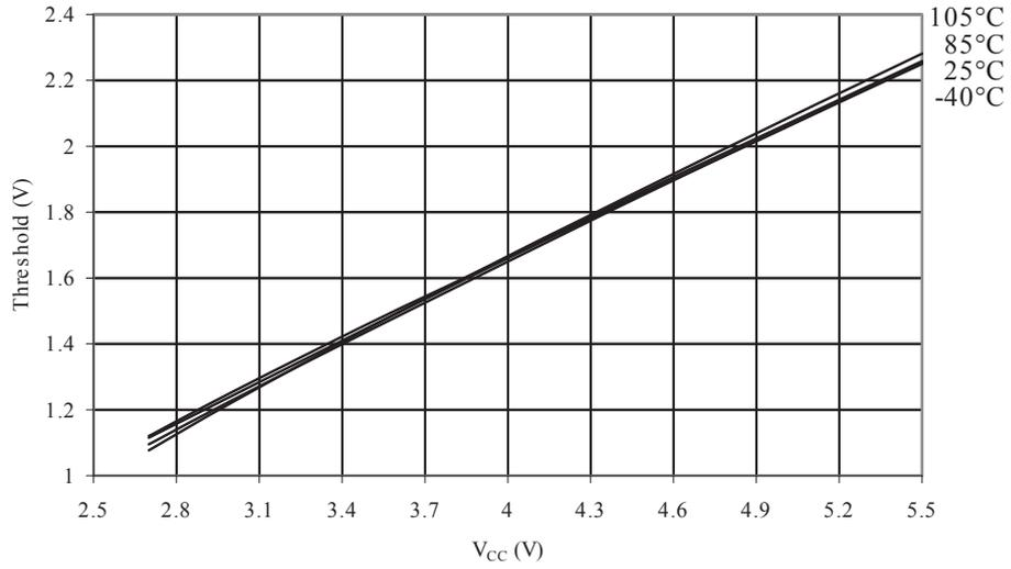
**Figure 35-25 I/O Pin Input Hysteresis vs.  $V_{CC}$**
