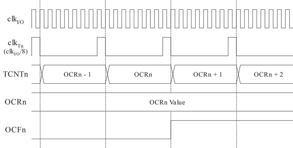
The next figure shows the setting of OCF2 and the clearing of TCNT2 in CTC mode.
