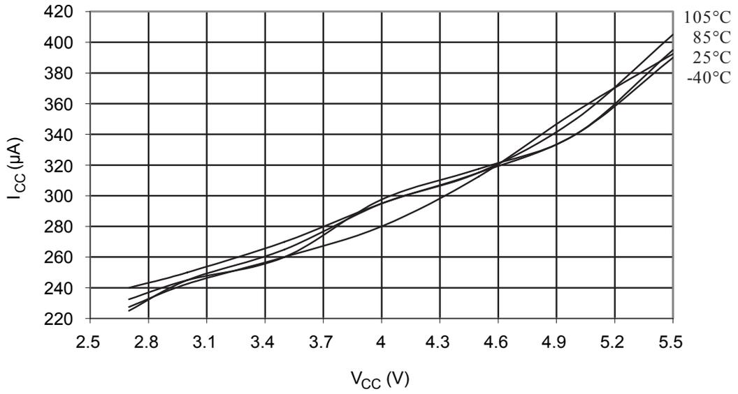
Figure 35-45 AREF External Reference Current vs.  $V_{CC}$
