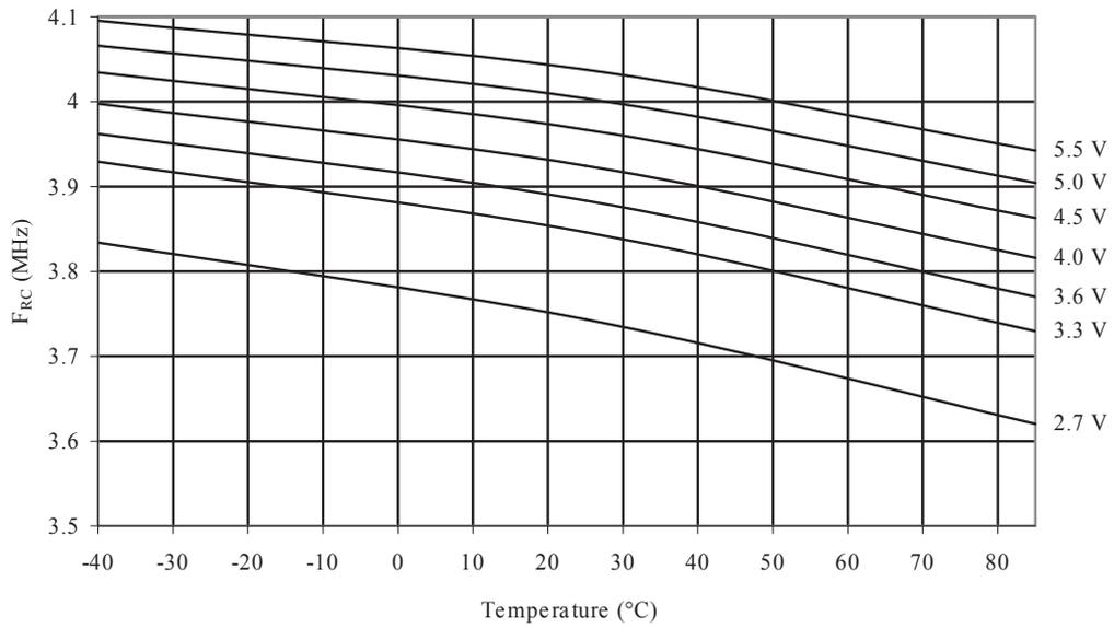
**Figure 34-47 Calibrated 4 MHz RC Oscillator Frequency vs.  $V_{CC}$**
