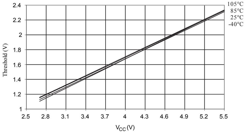
**Figure 35-28 Reset Input Pin Hysteresis vs. V<sub>CC</sub>**
