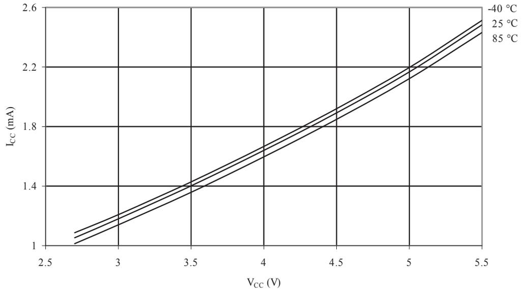
**Figure 34-13 Idle Supply Current vs.  $V_{CC}$  (Internal RC Oscillator, 8 MHz)**
