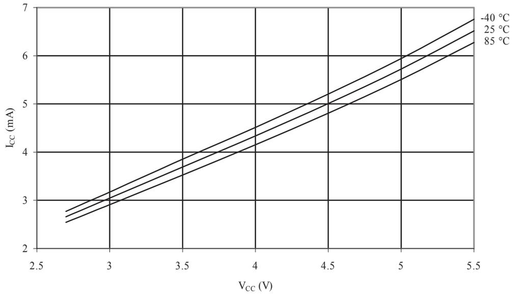
**Figure 34-6 Active Supply Current vs. V<sub>CC</sub> (Internal RC Oscillator, 8 MHz)**
