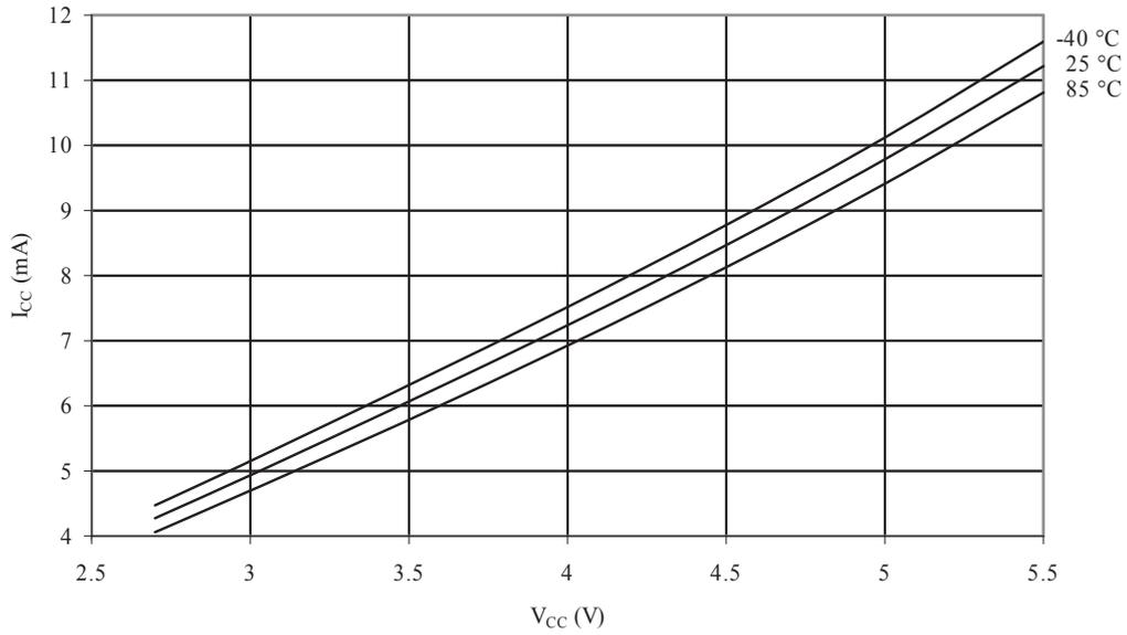
**Figure 34-7 Active Supply Current vs. V<sub>CC</sub> (32 kHz External Oscillator)**
