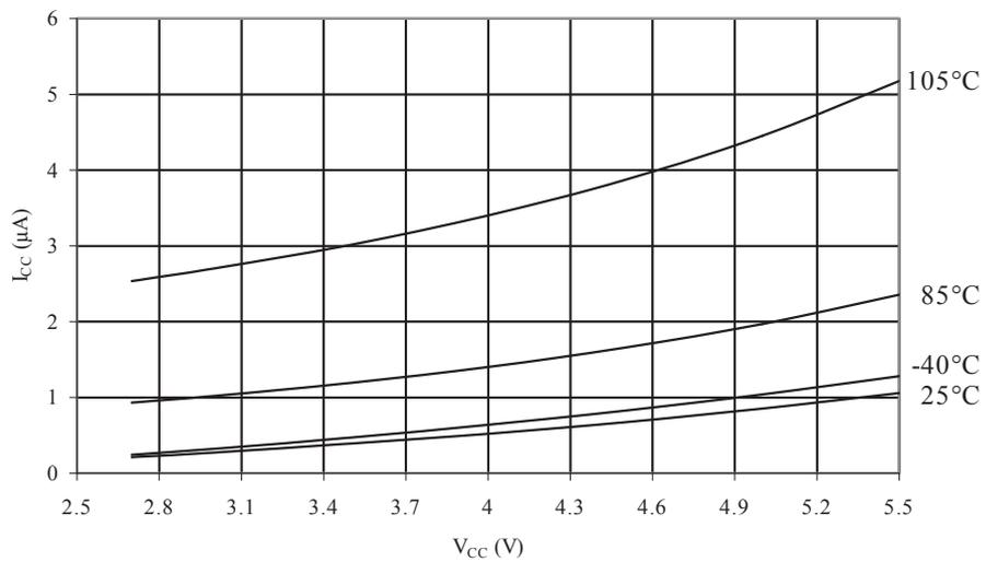
**Figure 35-14 Power-down Supply Current vs.  $V_{CC}$  (Watchdog Timer Enabled)**
