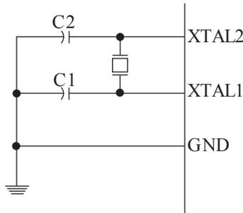
The Oscillator can operate in three different modes, each optimized for a specific frequency range. The operating mode is selected by the fuses CKSEL3:1 as shown in the following table.
