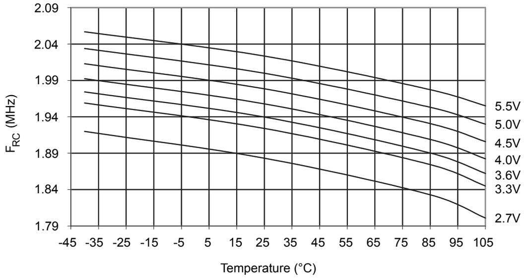
**Figure 35-37 Calibrated 2MHz RC Oscillator Frequency vs.  $V_{CC}$**
