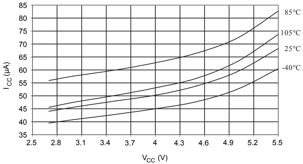
Figure 35-48 Programming Current vs.  $V_{CC}$
