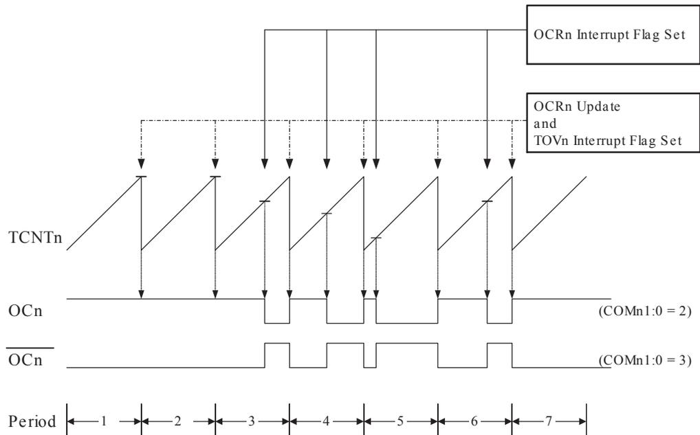
The Timer/Counter Overflow Flag (TOV0) is set each time the counter reaches MAX. If the interrupt is enabled, the interrupt handler routine can be used for updating the compare value.
