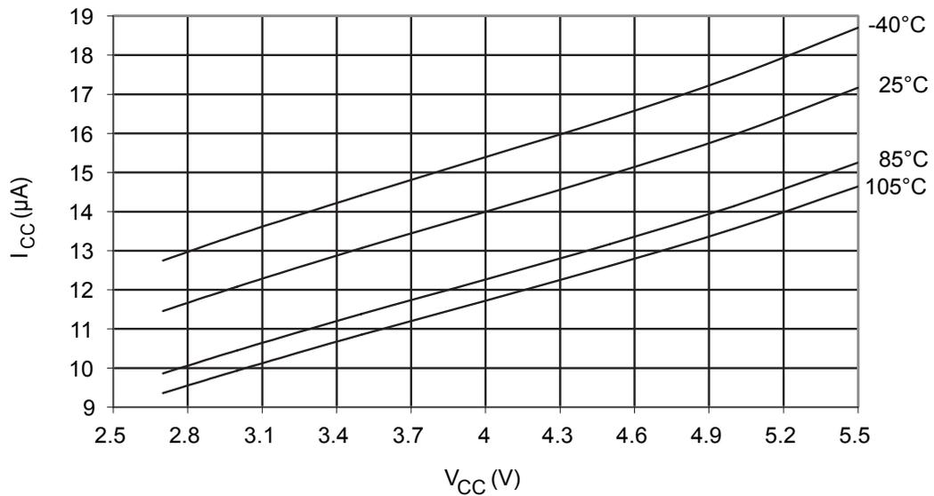
Figure 35-44 ADC Current vs.  $V_{CC}$  (AREF =  $AV_{CC}$ )
