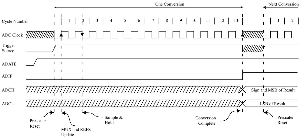
**Figure 28-7 ADC Timing Diagram, Free Running Conversion**
