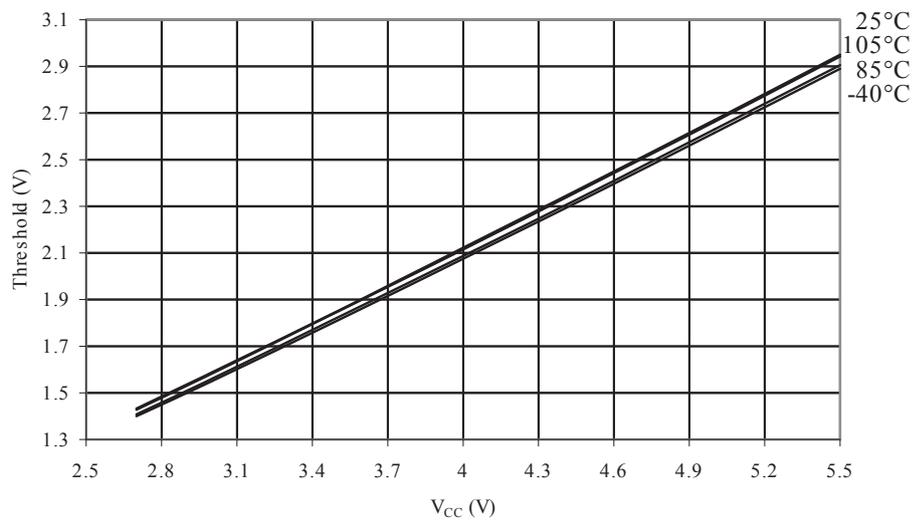
**Figure 35-24 I/O Pin Input Threshold Voltage vs.  $V_{CC}$  ( $V_{IL}$ , I/O Pin Read as "0")**
