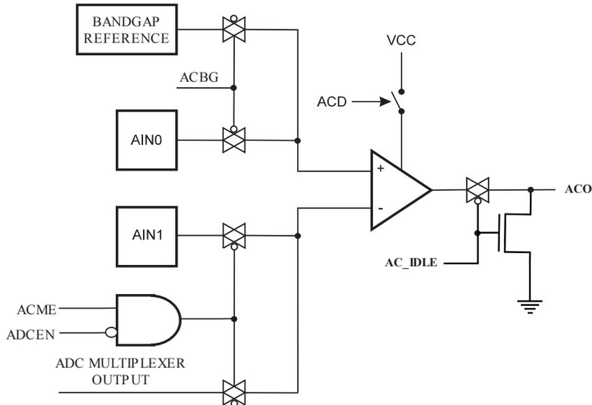
**Figure 29-11 General Boundary-scan Cell used for Signals for Comparator and ADC**
