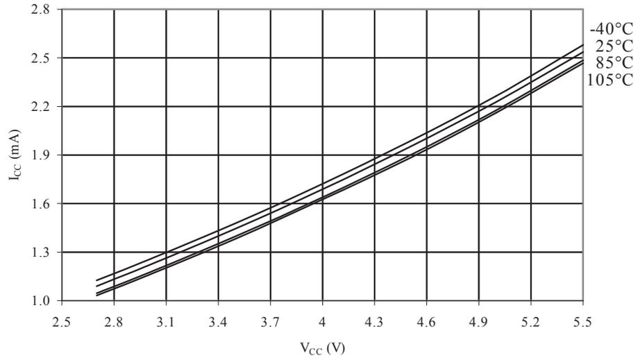
**Figure 35-11 Idle Supply Current vs. V<sub>CC</sub> (Internal RC Oscillator, 2MHz)**
