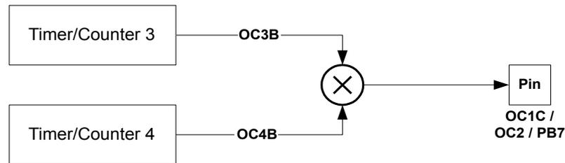
When the modulator is enabled, the two output compare channels are modulated together as shown in the block diagram above.
