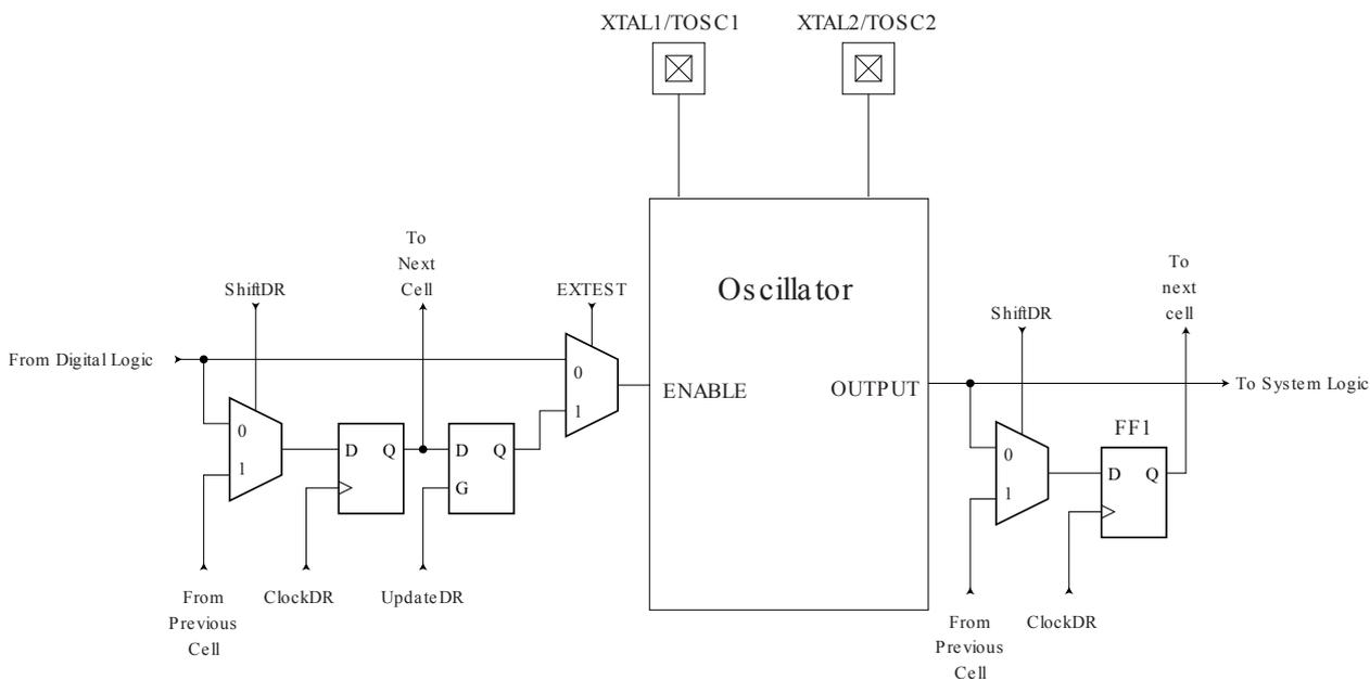
The following table summarizes the scan registers for the external clock pin XTAL1, oscillators with XTAL1/XTAL2 connections as well as 32kHz Timer Oscillator.
