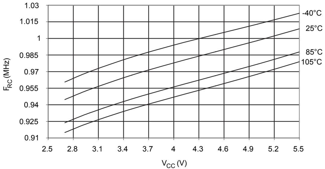
**Figure 35-36 Calibrated 2MHz RC Oscillator Frequency vs. Temperature**
