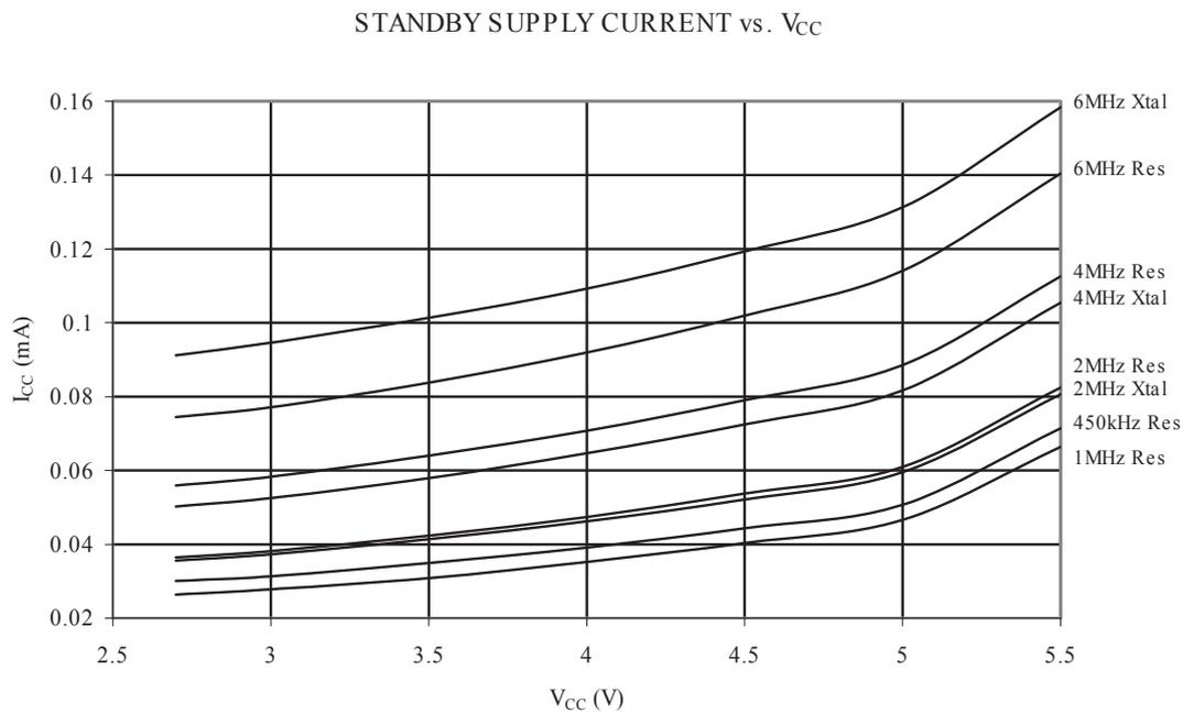
Figure 34-19 Standby Supply Current vs.  $V_{CC}$  (CKOPT Programmed)
