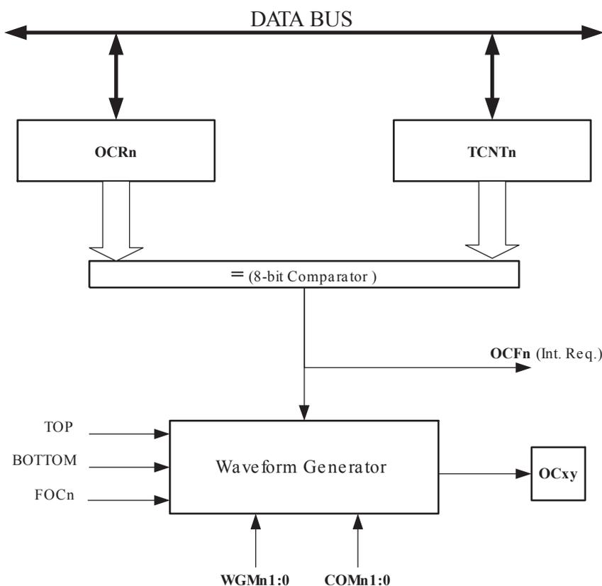
The OCR0 Register is double buffered when using any of the Pulse Width Modulation (PWM) modes. For the normal and Clear Timer on Compare (CTC) modes of operation, the double buffering is disabled. The double buffering synchronizes the update of the OCR0 Compare Register to either top or bottom of the counting sequence. The synchronization prevents the occurrence of odd-length, non-symmetrical PWM pulses, thereby making the output glitch-free.
