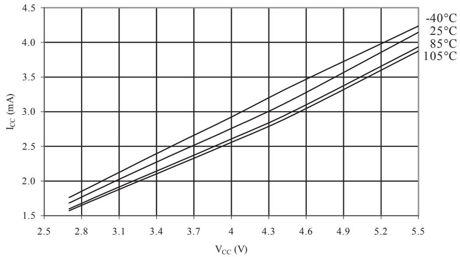
**Figure 35-6 Active Supply Current vs. V<sub>CC</sub> (Internal RC Oscillator, 1MHz)**
