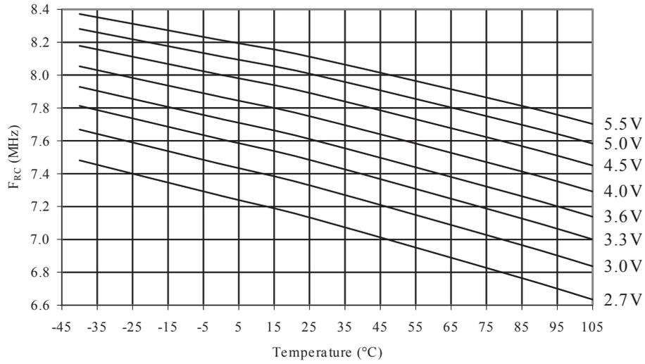
**Figure 35-41 Calibrated 8MHz RC Oscillator Frequency vs.  $V_{CC}$**
