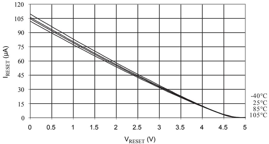
Figure 35-18 Reset Pull-up Resistor Current vs. Reset Pin Voltage (VCC = 2.7V)
