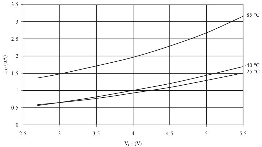
**Figure 34-16 Power-Down Supply Current vs. V<sub>CC</sub> (Watchdog Timer Enabled)**
