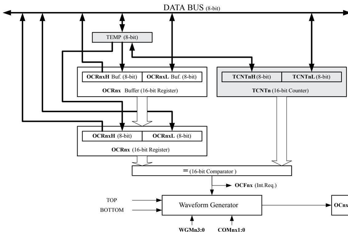
The OCRnx Register is double buffered when using any of the twelve *Pulse Width Modulation* (PWM) modes. For the normal and *Clear Timer on Compare* (CTC) modes of operation, the double buffering is disabled. The double buffering synchronizes the update of the OCRnx Compare Register to either TOP or BOTTOM of the counting sequence. The synchronization prevents the occurrence of odd-length, non-symmetrical PWM pulses, thereby making the output glitch-free.
