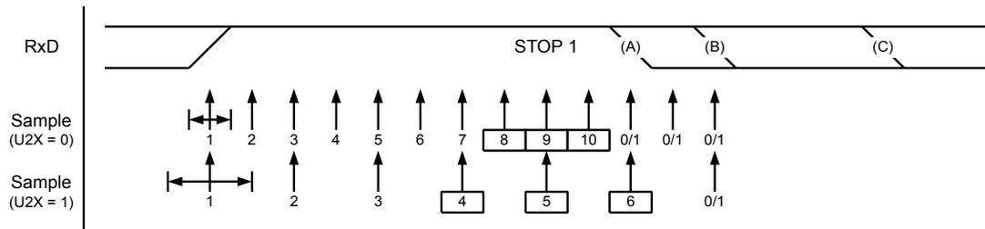
The same majority voting is done to the stop bit as done for the other bits in the frame. If the stop bit is registered to have a logic 0 value, the Frame Error (FE) Flag will be set.
