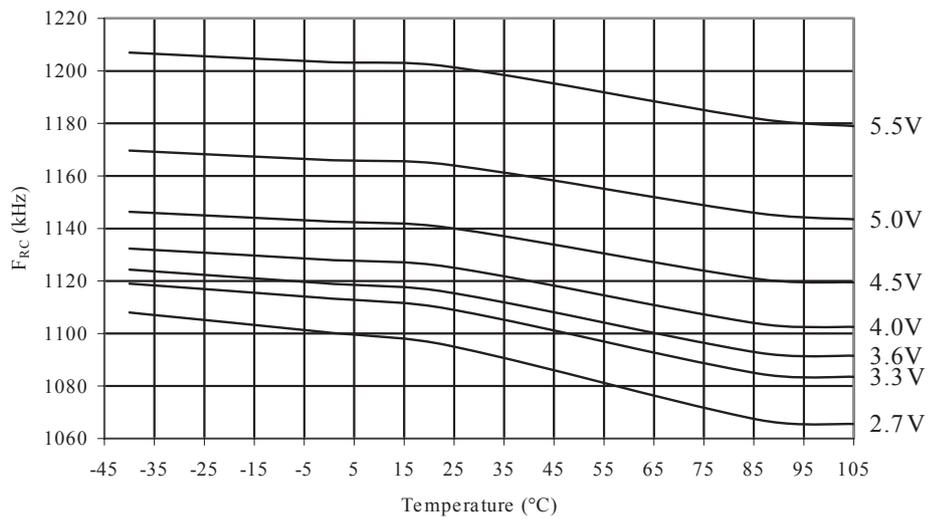
**Figure 35-34 Calibrated 1MHz RC Oscillator Frequency vs. Temperature**
