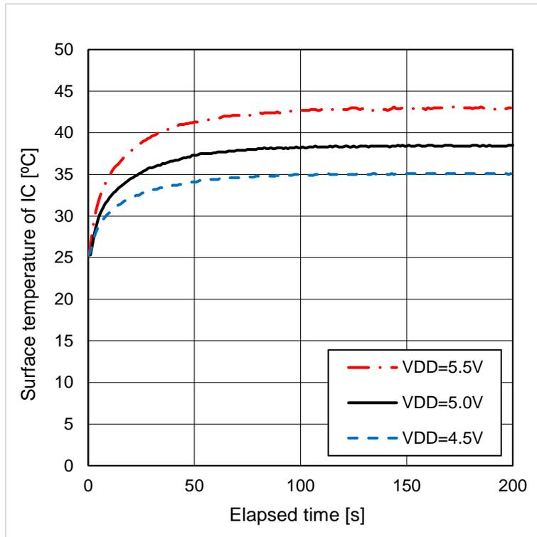
Figure 4. Surface temperature of IC vs Elapsed time
