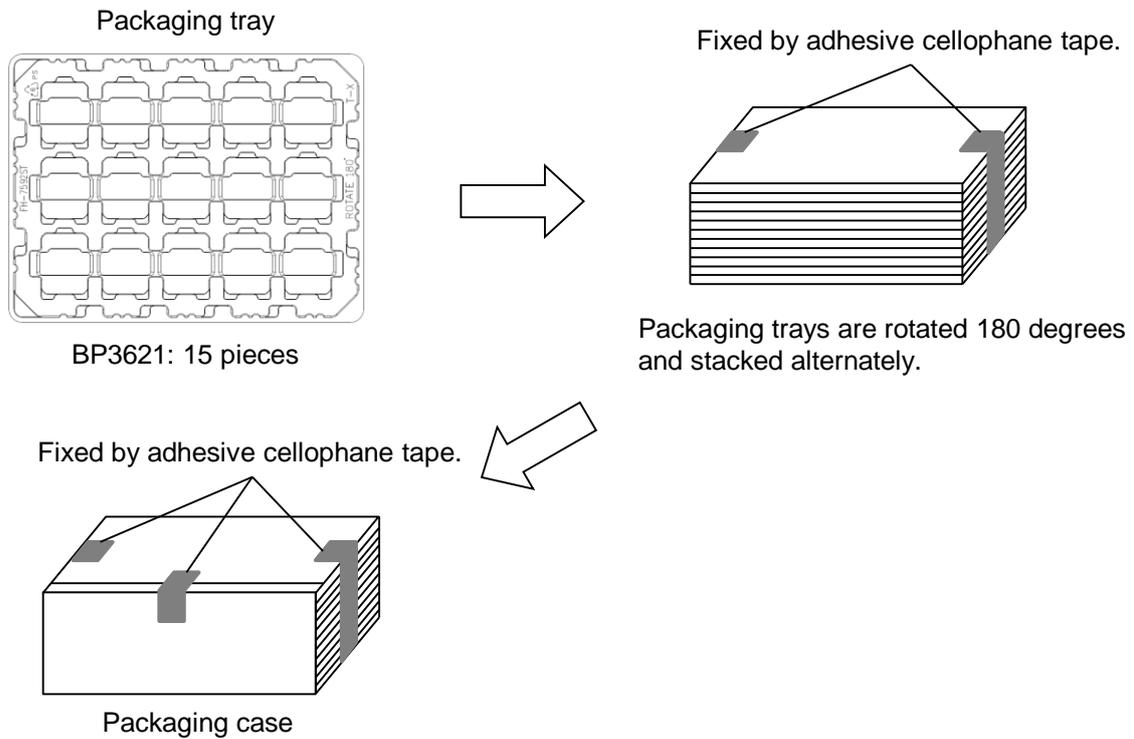
Figure 12. Packing Method
