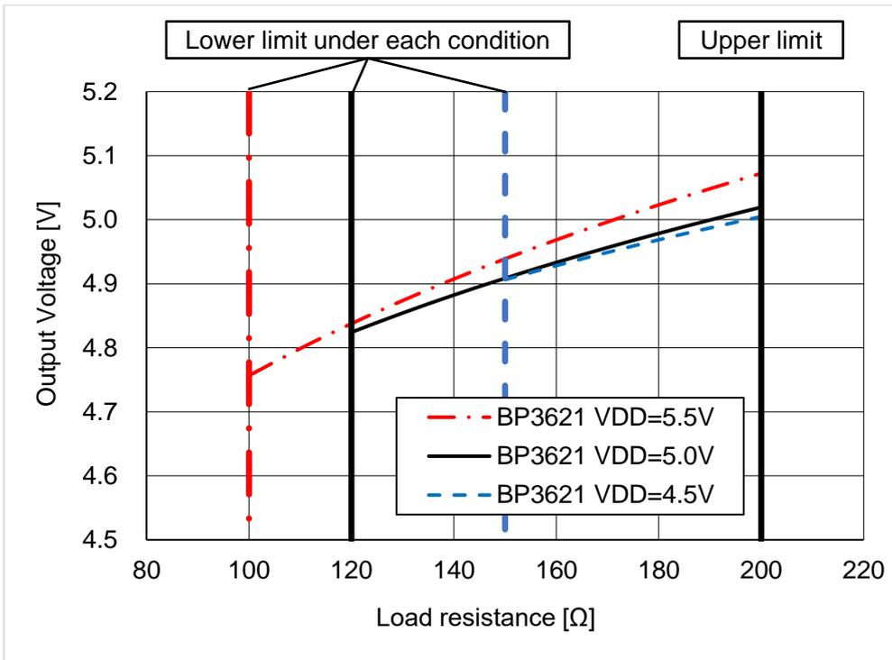
Figure 3. Output Voltage vs Load resistance
