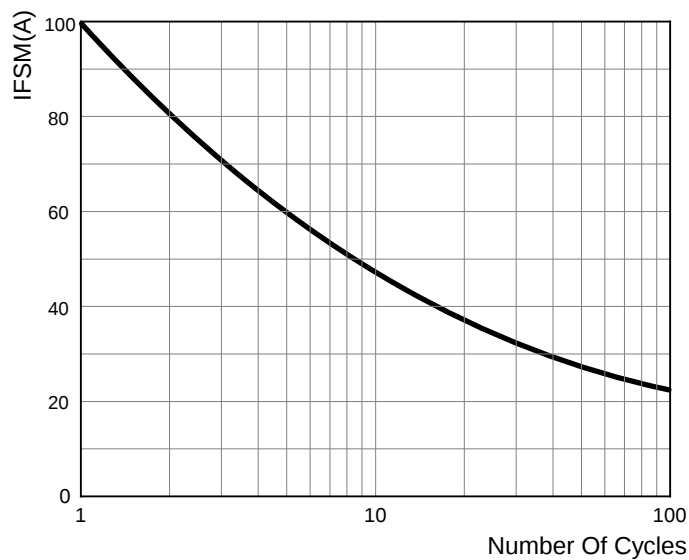
FIG 2: MAXIMUM NON-REPETITIVE FORWARD SURGE CURRENT
