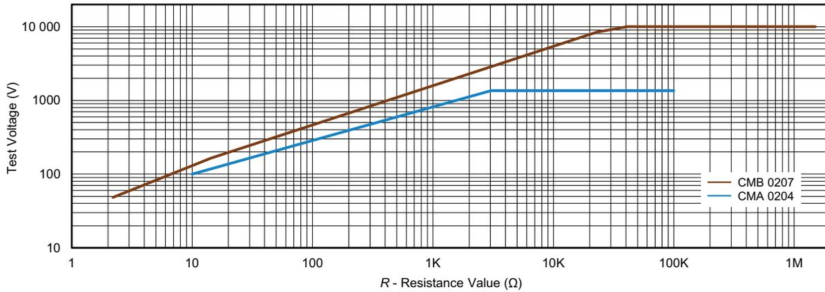
Pulse load rating in accordance with IEC 60115-1, clause 4.27; 10 μs / 700 μs; 10 pulses at 1 minute intervals; for permissible resistance change ± (0.5 % R + 0.05 Ω)
