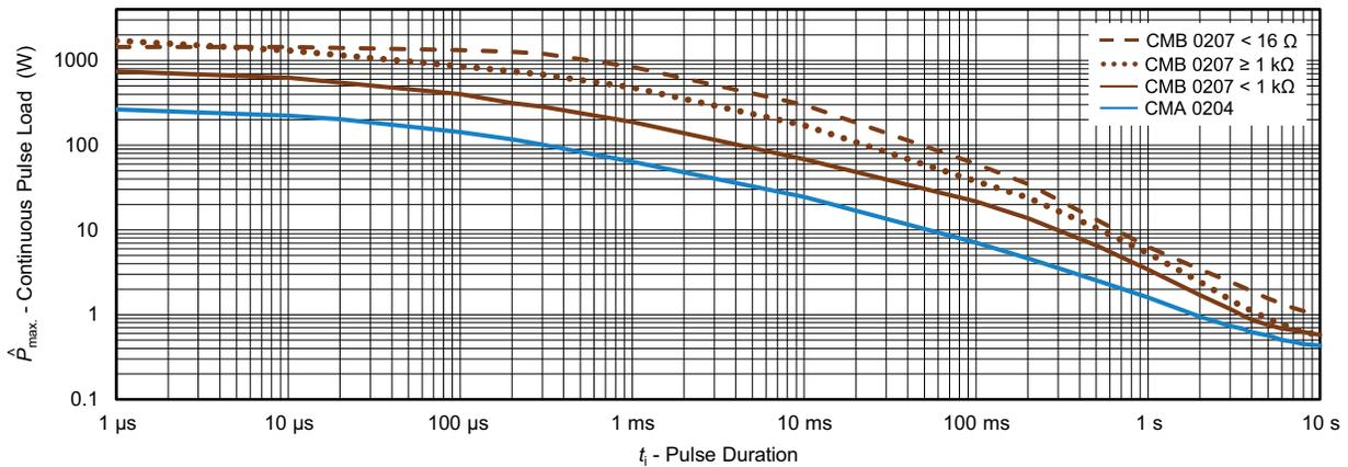
Maximum pulse load, continuous pulse; applicable if  $\bar{P} \leq P(\vartheta_{amb})$  and  $\hat{U} \leq 4$  kV (CMB); or  $\hat{U} \leq 2$  kV (CMA); for permissible resistance change  $\pm (0.5 \% R + 0.01 \Omega)$
