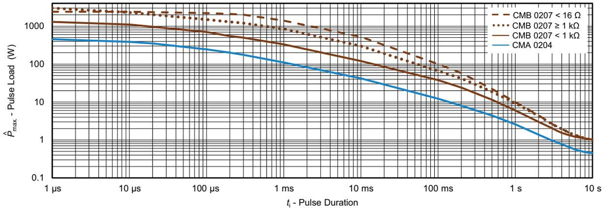
Maximum pulse load, single pulse; applicable if  $\bar{P} \rightarrow 0$  and  $n \leq 1000$  and  $\hat{U} \leq 4$  kV (CMB); or  $\hat{U} \leq 2$  kV (CMA); for permissible resistance change  $\pm (0.5 \% R + 0.01 \Omega)$
