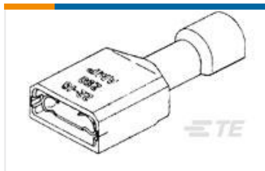
TE Part #3-520140-2 ULTRA-FAST 250 ASY REC 16-14 AWG TPBR
