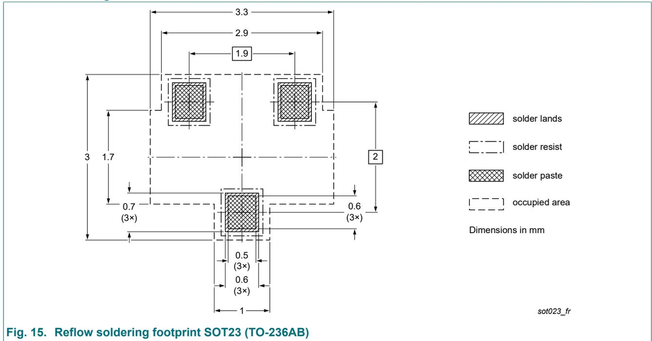
Fig. 15. Reflow soldering footprint SOT23 (TO-236AB)
