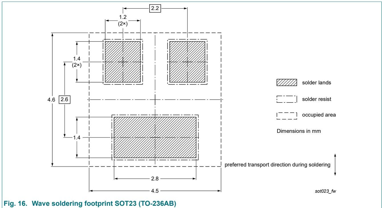
Fig. 16. Wave soldering footprint SOT23 (TO-236AB)
