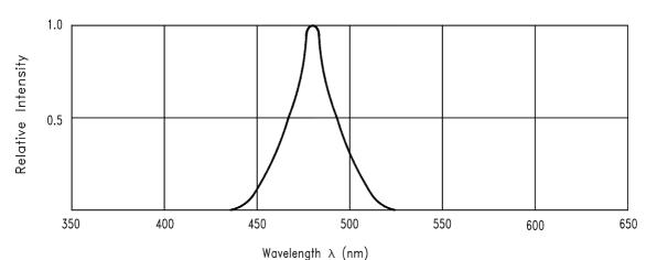
Fig.1 Relative Intensity vs. Wavelength
