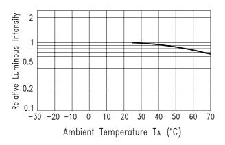
Fig.5 Luminous Intensity vs.
