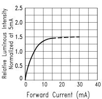
Fig.4 Relative Luminous Intensity vs. Forward Current
