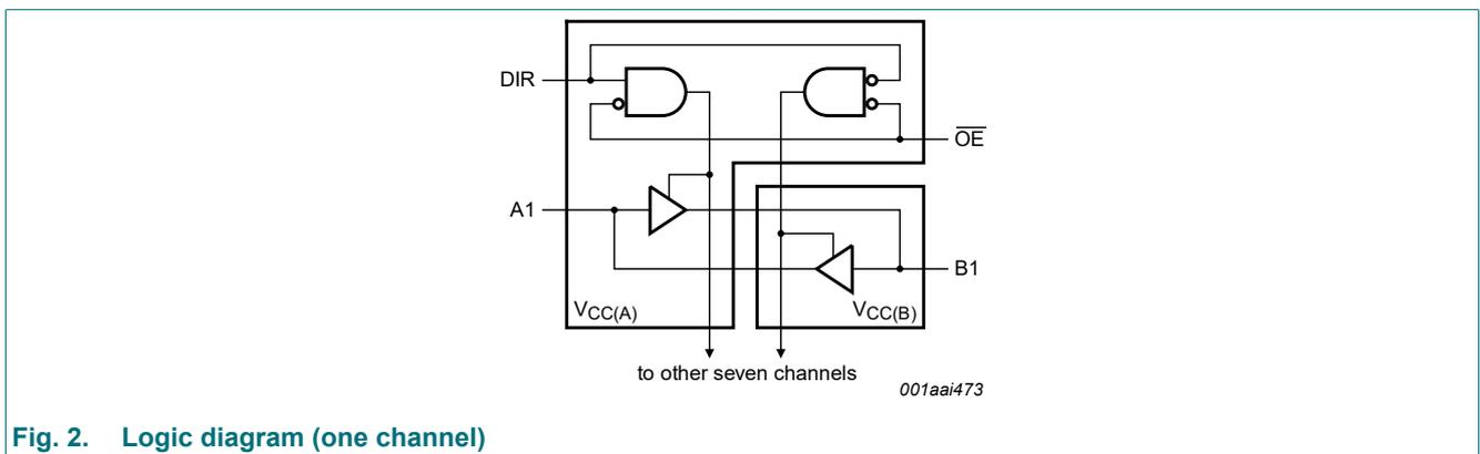
Fig. 2. Logic diagram (one channel)
