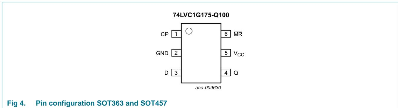
Fig 4. Pin configuration SOT363 and SOT457
