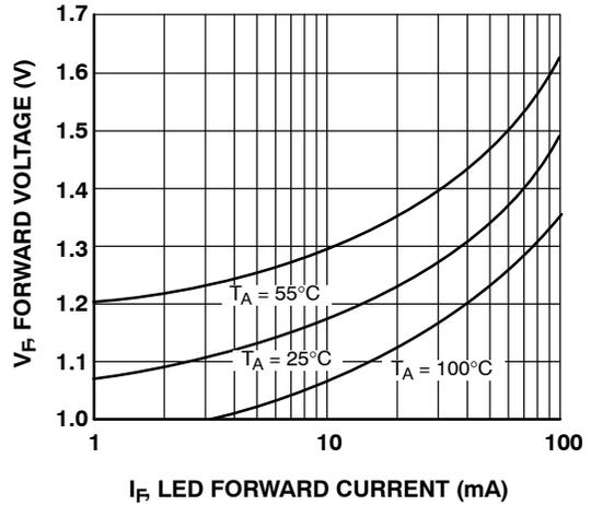
Figure 6. LED Forward Voltage vs. Forward Current
