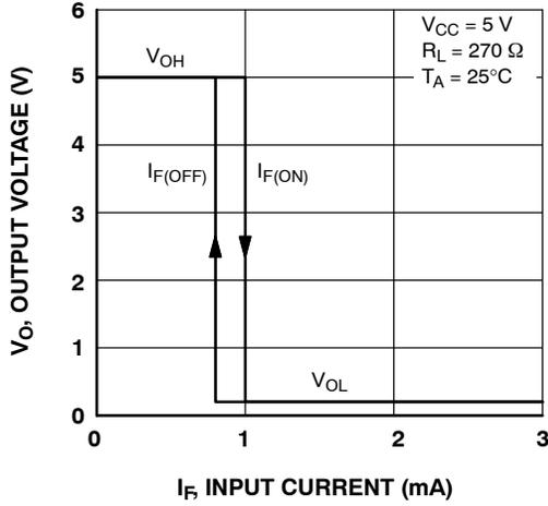
Figure 1. Transfer Characteristics
