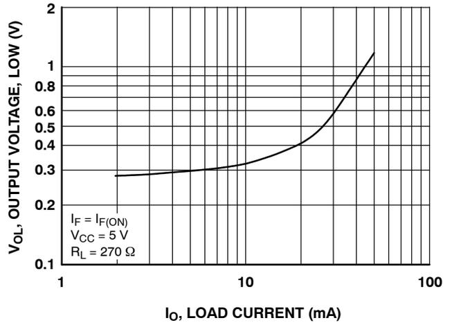
Figure 4. Output Voltage, Low vs. Load Current
