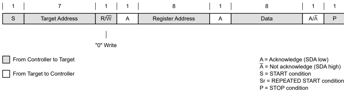
Figure 9-19. "Write" Data Transfer Format in Standard, Fast, Fast Plus Modes
