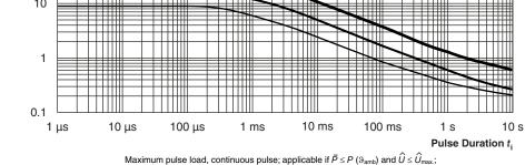
for permissible resistance change  $\pm$  (0.5 % *R* + 0.01  $\Omega$ ) Continuous Pulse for *R* < 10  $\Omega$
