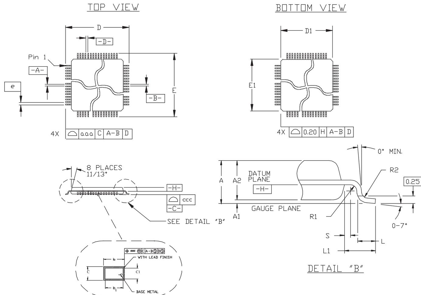
Table 11-1. 208-lead PQFP Package Dimensions (in mm)
