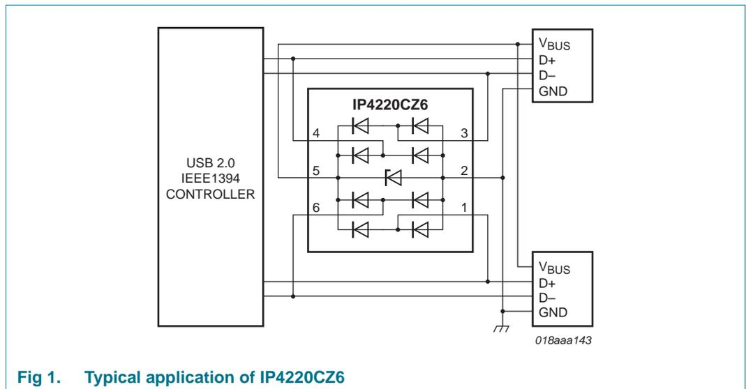
**Fig 1. Typical application of IP4220CZ6**
