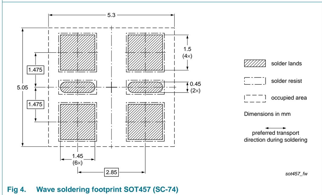
Fig 4. Wave soldering footprint SOT457 (SC-74)
