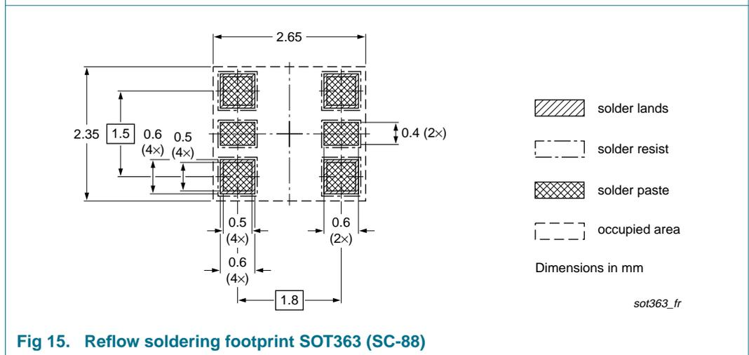
Fig 15. Reflow soldering footprint SOT363 (SC-88)
