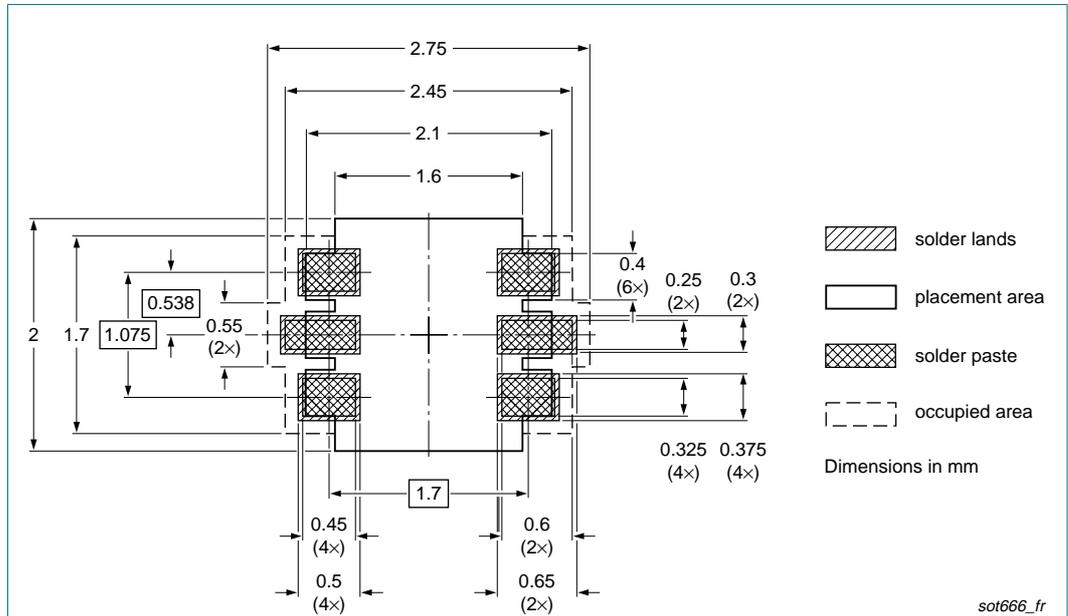
Reflow soldering is the only recommended soldering method.
