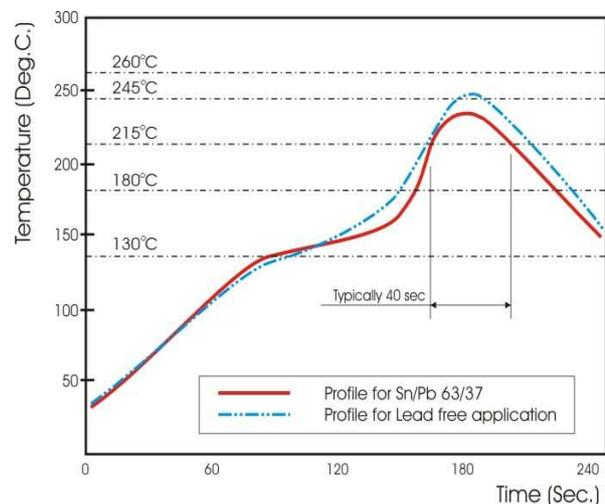
Fig 3. Infrared soldering profile for Chip Resistors WR02X(W)
