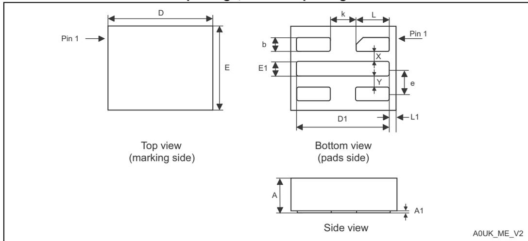
1. On the bottom side, pin 1 is identified by the specific pad shape and, on the top side, pin 1 is defined from the orientation of the marking: when reading the marking, pin 1 is below the upper left package corner.
