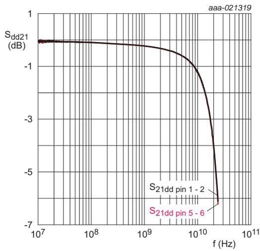
Fig 1. Differential mode insertion loss; typical values
