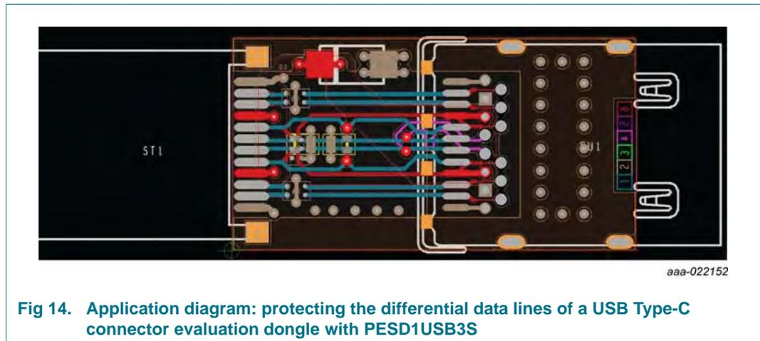
Since the SuperSpeed TX/RX lines are separated by GND or VBUS from the Hi-Speed lines, PESD1USB3S makes it easy to achieve same signal lengths, straight routing, and optimal positioning for ESD protection directly at the connector.
