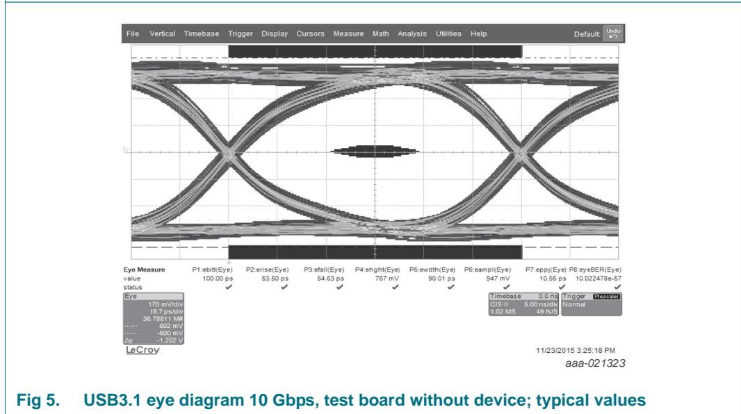
Fig 5. USB3.1 eye diagram 10 Gbps, test board without device; typical values
