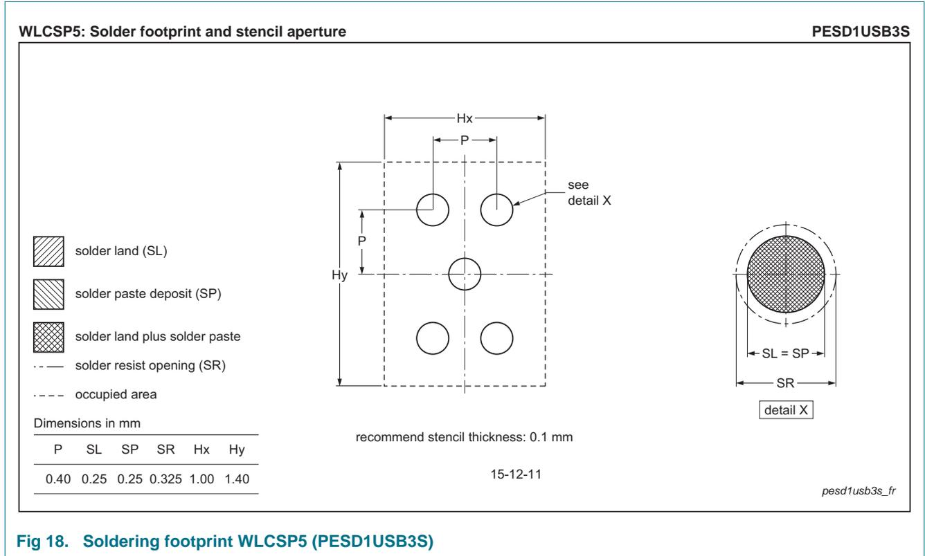
**Fig 18. Soldering footprint WLCSP5 (PESD1USB3S)**
