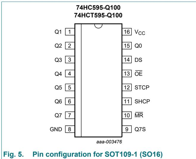
Fig. 5. Pin configuration for SOT109-1 (SO16)
