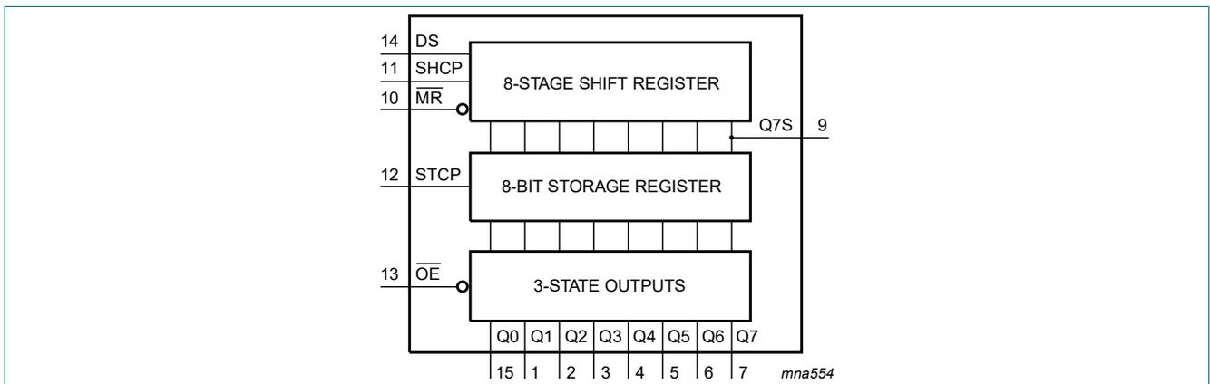
Fig. 1. Functional diagram
