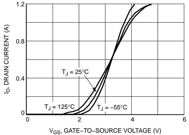
Figure 2. Transfer Characteristics
