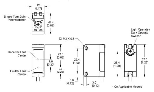
Maximum mounting screw torque: 0.56 Nm (5 in-lbs)
