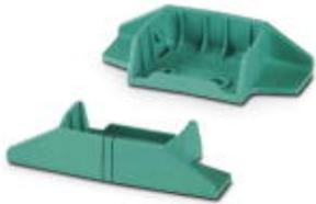
Stand for mounting the UCS housing, height: 47 mm; material: polyamide; color: turquoise blue, similar to RAL 5018; wall mounting option is integrated, snaps into the screw holes of the housing
