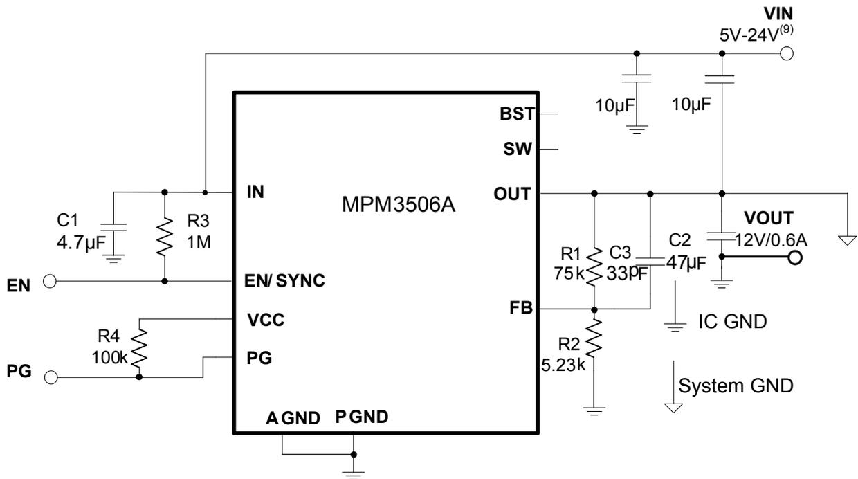
Figure 15:  $V_{OUT} = -12V$ ,  $I_{OUT} = 0.6A$
