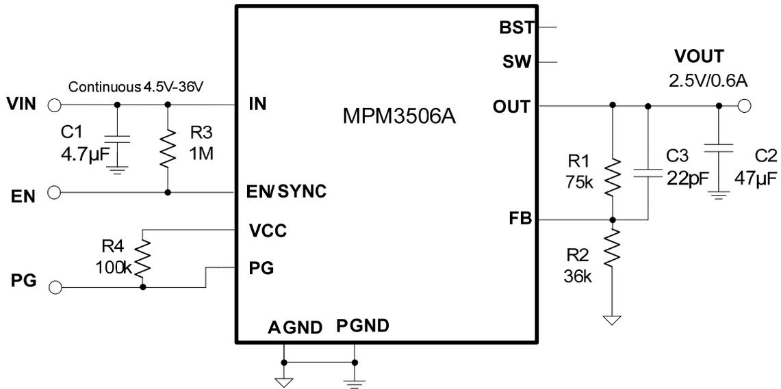
Figure 10:  $V_{OUT} = 2.5V$ ,  $I_{OUT} = 0.6A$
