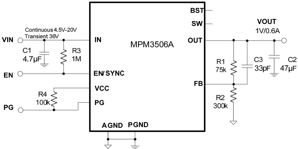
Figure 14:  $V_{OUT} = 1V$ ,  $I_{OUT} = 0.6A$
