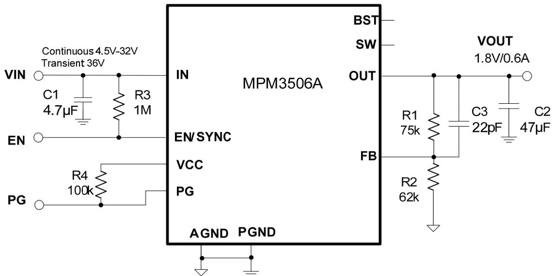
Figure 11:  $V_{OUT} = 1.8V$ ,  $I_{OUT} = 0.6A$
