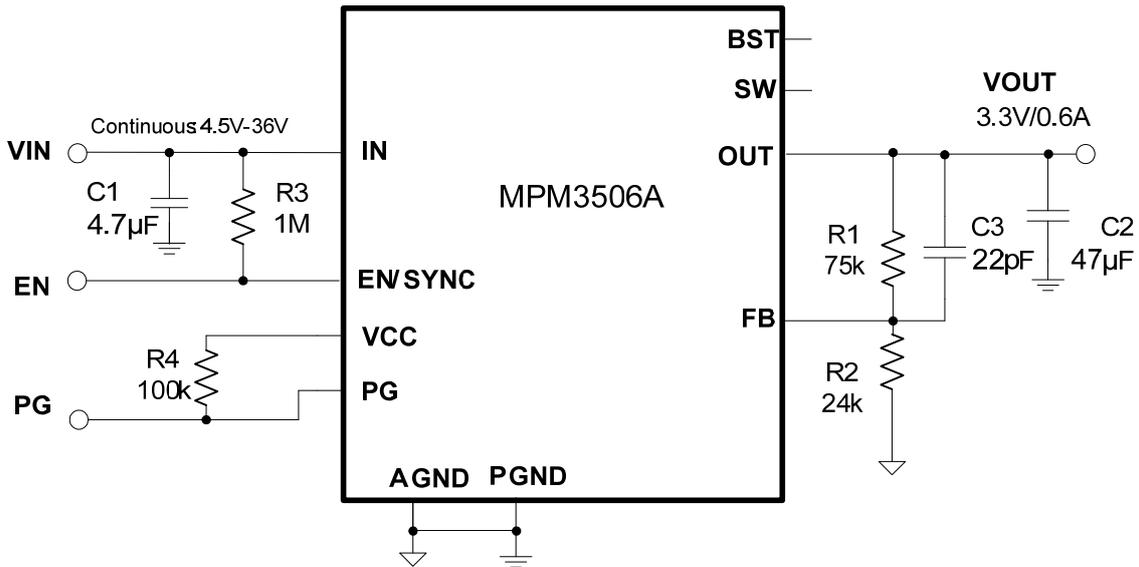
Figure 9:  $V_{OUT} = 3.3V$ ,  $I_{OUT} = 0.6A$
