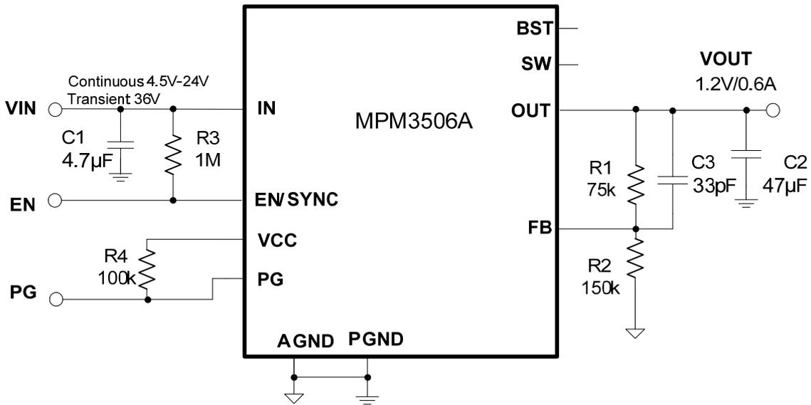
Figure 13:  $V_{OUT} = 1.2V$ ,  $I_{OUT} = 0.6A$
