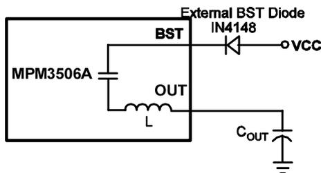
**Figure 6: Optional External Bootstrap Diode to Enhance Efficiency**
