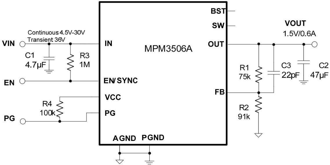
Figure 12:  $V_{OUT} = 1.5V$ ,  $I_{OUT} = 0.6A$
