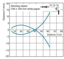
Sensing Distance vs. Material Diffuse-reflective
