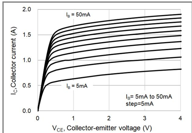
Fig.12 Collector Current (-40)
