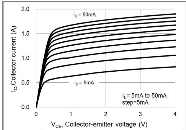
Fig.10 Collector Current (-16)
