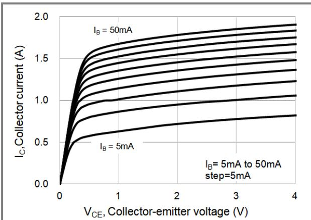
Fig.11 Collector Current (-25)
