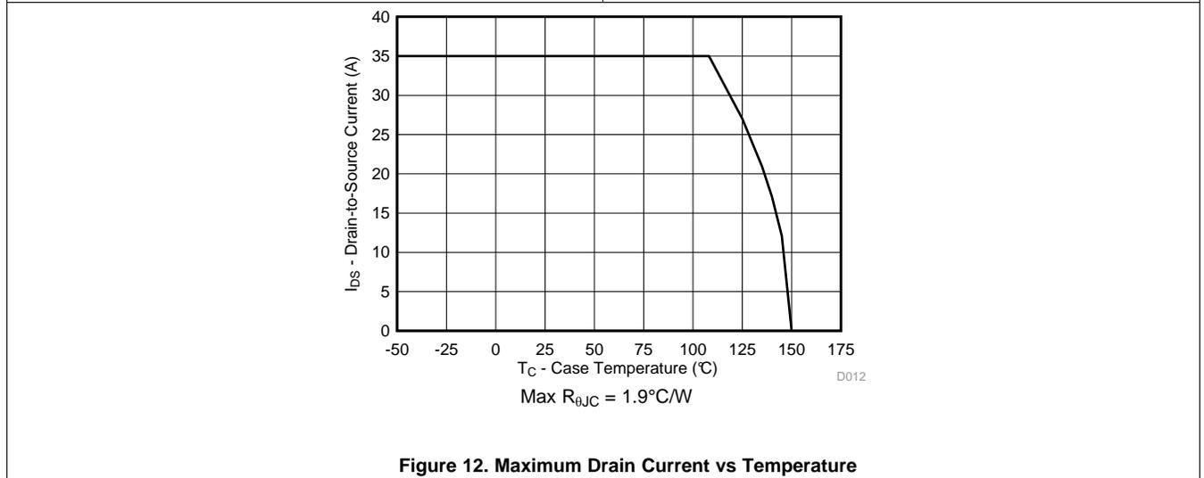
Figure 12. Maximum Drain Current vs Temperature
