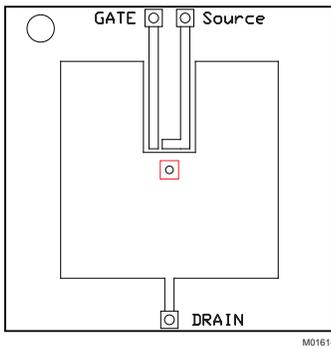
Max  $R_{\theta JA} = 55^{\circ}\text{C/W}$
