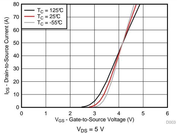
Figure 3. Transfer Characteristics
