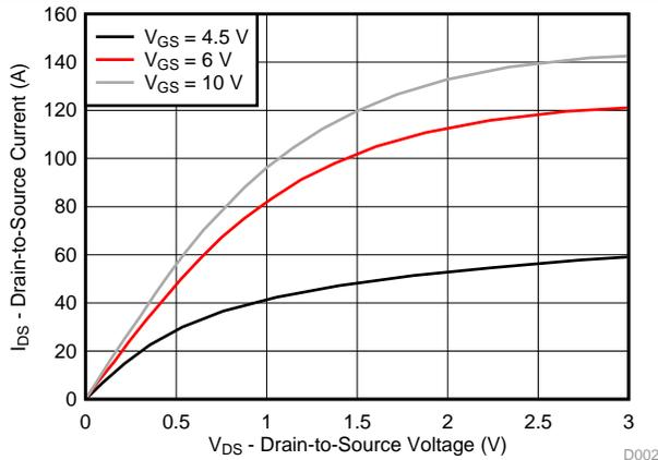
Figure 2. Saturation Characteristics
