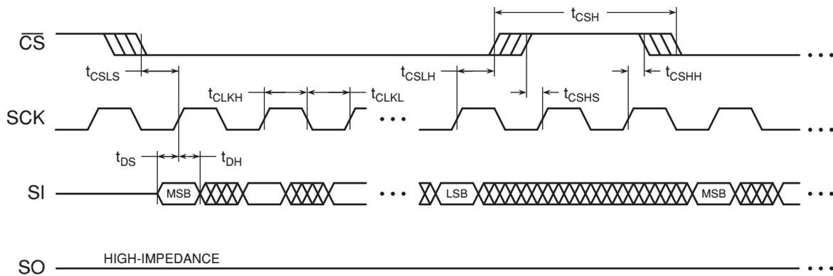
Figure 15-2. Serial Output Timing
