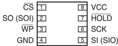
Figure 2-2. 8-UDFN (Top View)
