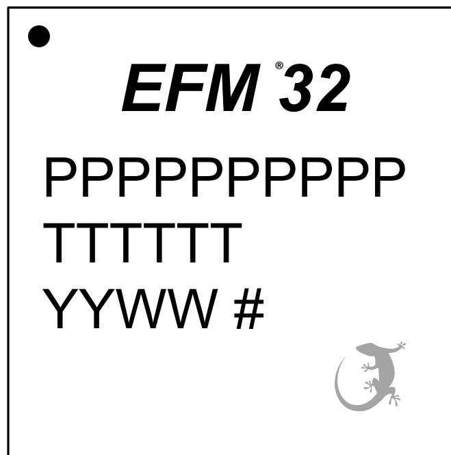
Figure 8.3. QFN40 Package Marking
