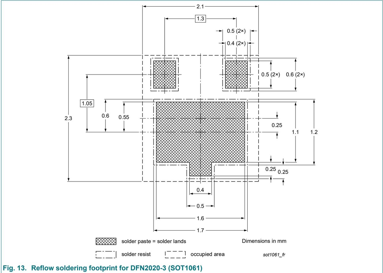
**Fig. 13. Reflow soldering footprint for DFN2020-3 (SOT1061)**
