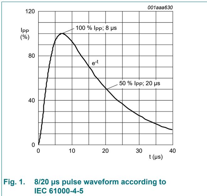
**Fig. 1. 8/20 μs pulse waveform according to IEC 61000-4-5**
