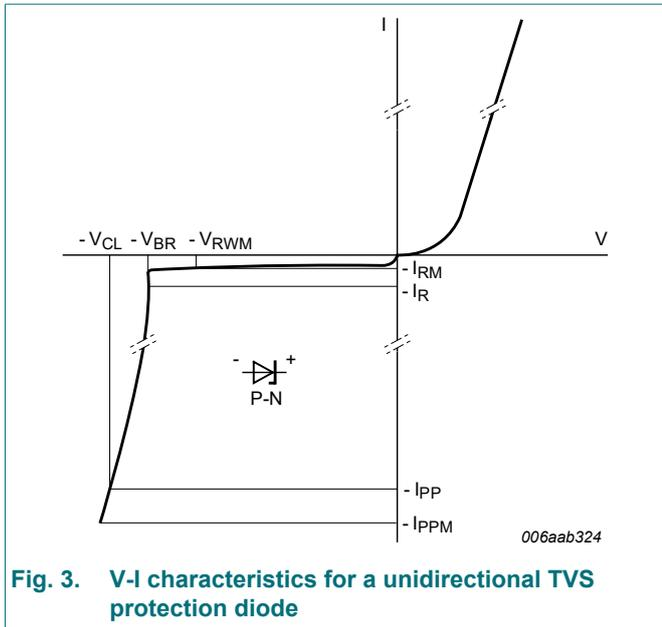
Fig. 3. V-I characteristics for a unidirectional TVS protection diode
