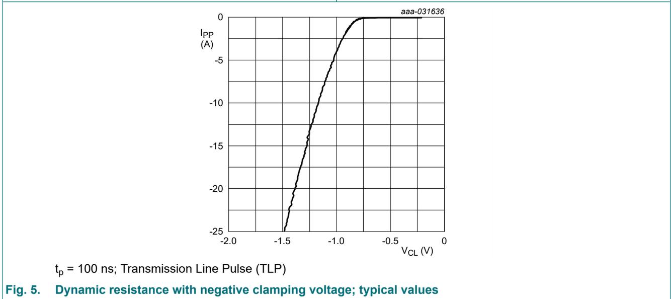
Fig. 5. Dynamic resistance with negative clamping voltage; typical values
