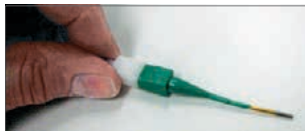
Plastic tool with contact in proper position.
