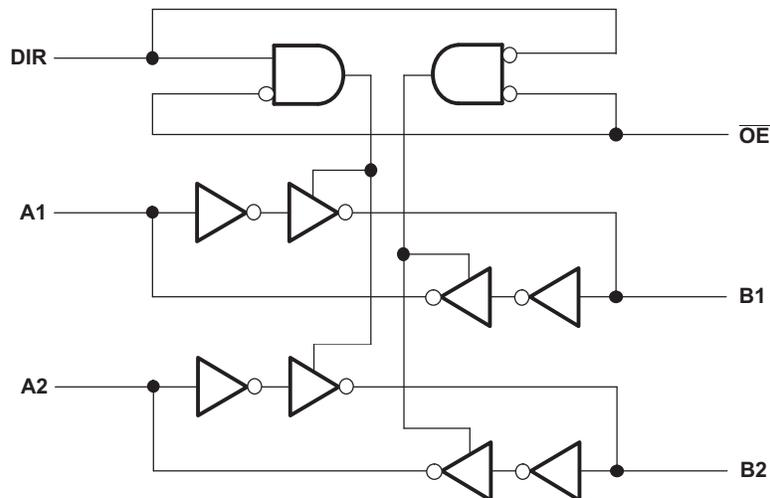
Figure 4. Logic Diagram (Positive Logic) for 1/2 of SN74AVC4T245
