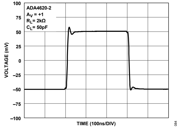
Figure 83. ADA4620-2 Small Signal Transient Response (100 mV Step, A_V = +1 )
