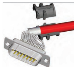
Attach the strain relief around the cable
