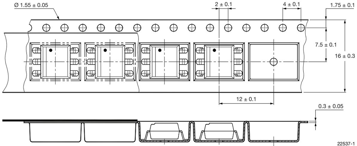
Fig. 16 - Tape and Reel Drawing, 1000 Units per Reel
