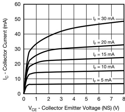
Fig. 6 - Collector Current vs. Collector Emitter Voltage (NS)
