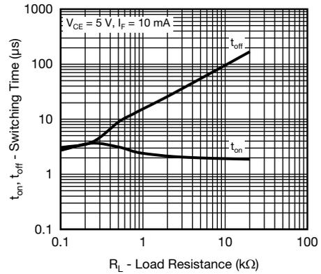
Fig. 15 - Switching Time vs. Load Resistance
