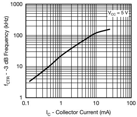
Fig. 14 - CTR -3 dB Frequency vs. Collector Current
