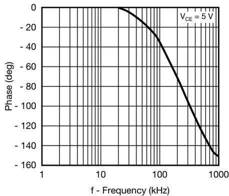
Fig. 13 - CTR Frequency vs. Phase Angle
