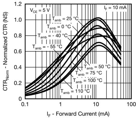
Fig. 11 - Normalized CTR (NS) vs. Forward Current
