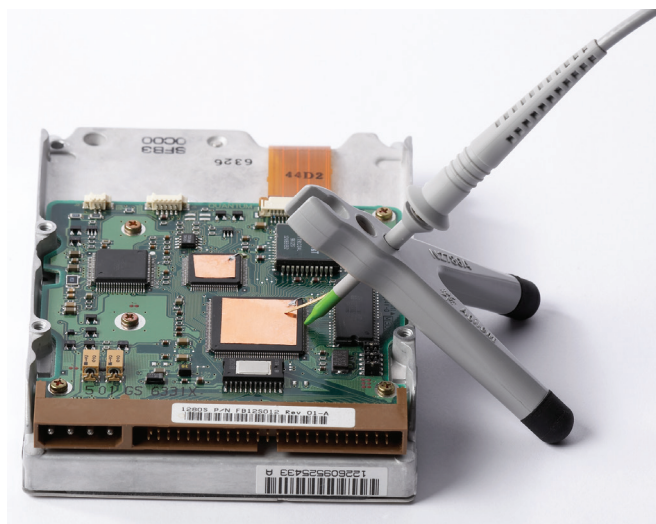
Figure 8. An IC cap adapter and ground blade with optional N2876A two-leg probe positioner offers an ideal hands-free solution for short circuit-proof probing of a fine-pitch IC. The N2877A deluxe accessory kit and N2878A fine-pitch accessory kit contain one N2876A two-leg probe positioner.
