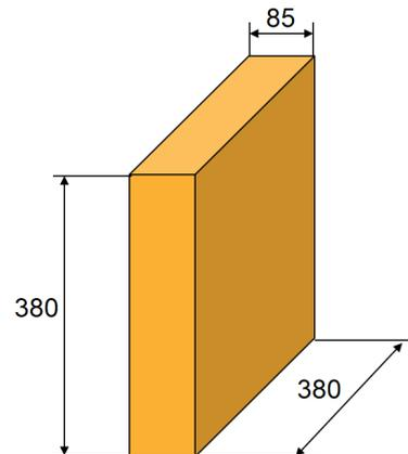
Figure 18. Ammopack dimension values (mm)
