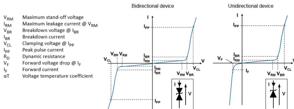
Figure 2. Pulse definition for electrical characteristics
