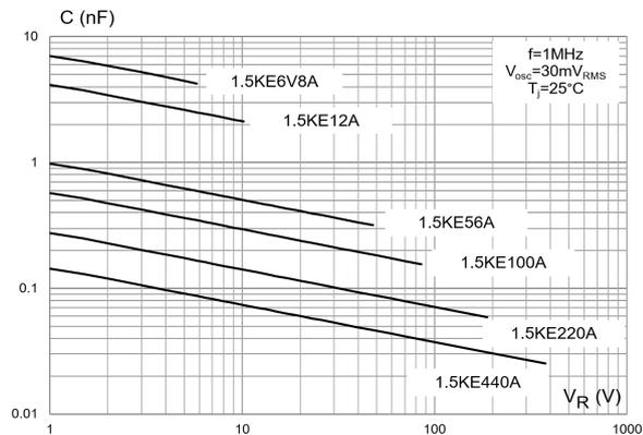
**Figure 8. Junction capacitance versus applied voltage (bidirectional type)**
