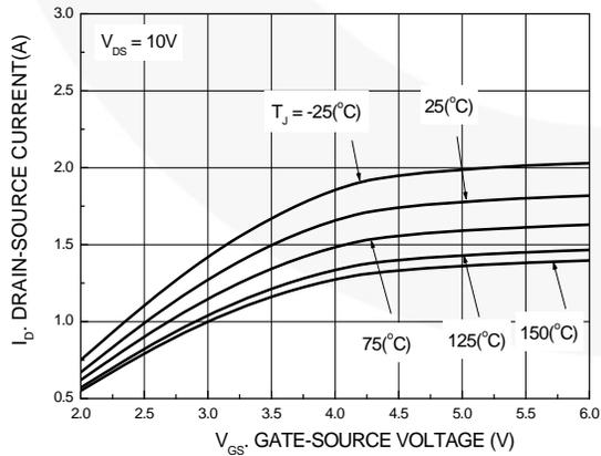
**Figure 5. Transfer Characteristics**
