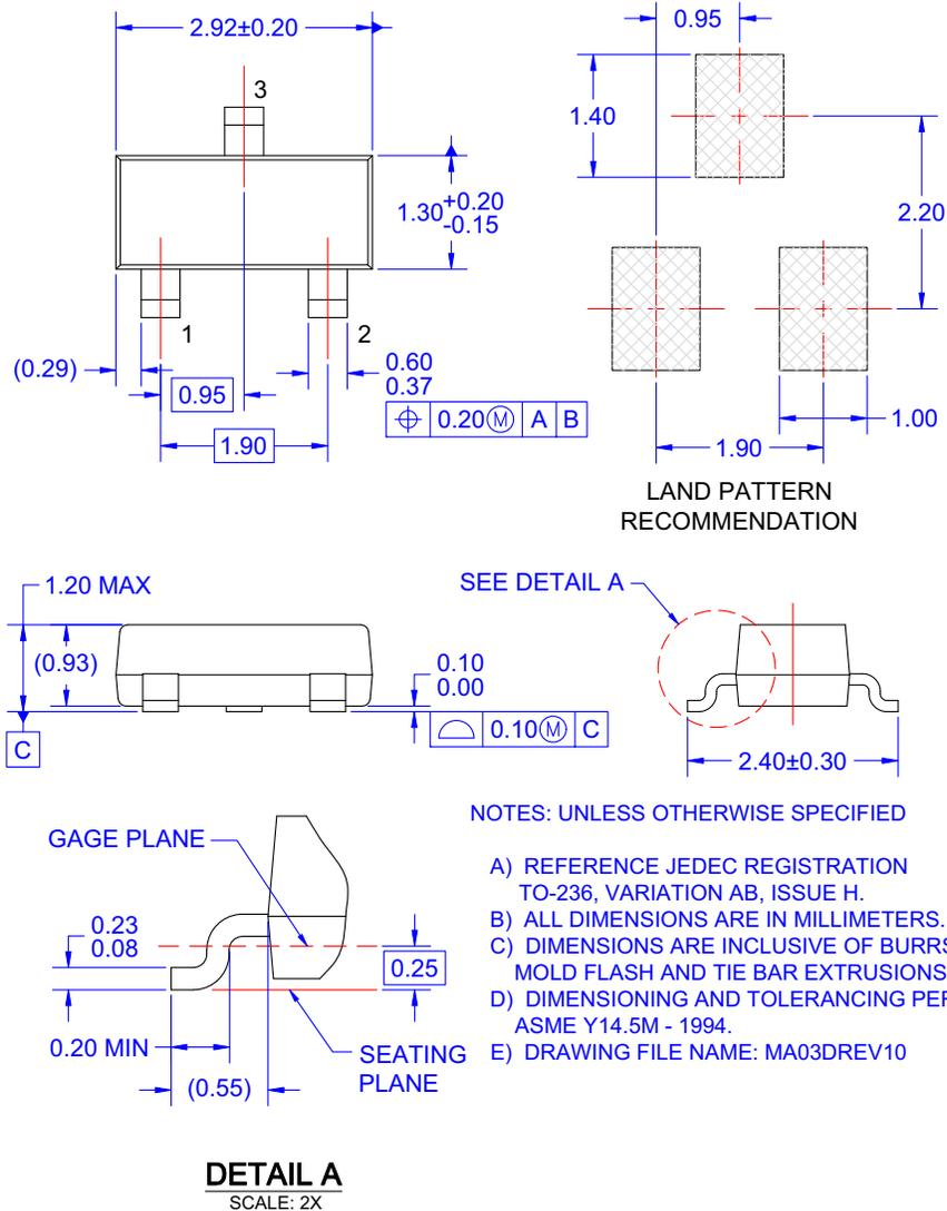
**Figure 8. 3LEAD, SOT23, JEDEC TO-236, LOW PROFILE (ACTIVE)**
